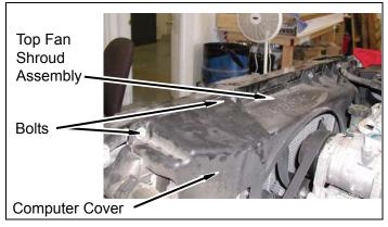
f. Install two kit washers (1/2" USS) as spacers inbetween upper fan shroud and computer cover as shown.
