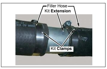
e. Install filler hose on fuel tank with clamp.
