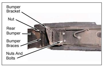
d. Install two kit **brackets** (rear bumper) on rear bumper with four bolts and nuts. Do not tighten.
