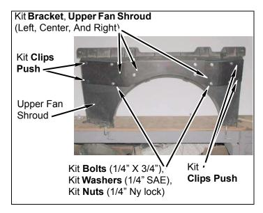
j. Using kit bracket, upper fan shroud (center) as template, drill two 1/4" holes in fan shroud lip. Install kit bracket, upper fan shroud (center) on upper fan shroud lip with two kit clips push.
