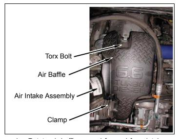
b. Rotate air baffle up and forward from intake as shown and loosen clamp.
