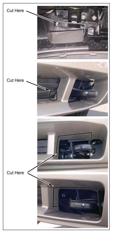
g. **2005 GMC models:** Repeat above step for passenger side front bumper. Check fitment and trim driver and passenger side, if necessary.
