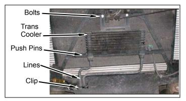
b. Remove two transmission cooler lines from clip.
