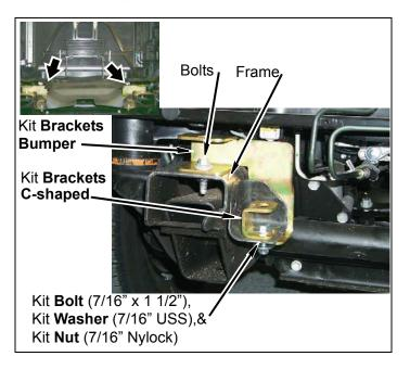
e. **2003-2004 models:** Mark and cut two front bumper brackets. Bend bottom edge of bumper bracket up toward bumper.
