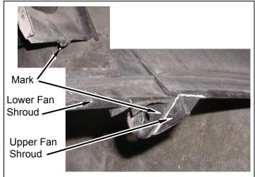
b. Measure upper fan shroud from top down1-1/2". Mark and cut upper fan shroud as shown.
