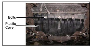
b. Remove plastic cover from push clip, lower radiator hose and vehicle.
