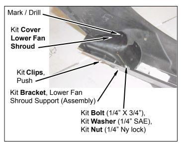
m. Using kit **cover** lower fan shroud as a template drill three 1/4" holes in lower fan shroud.
