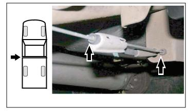
Separate front parking brake cable from rear parking brake cable at cable connector.
