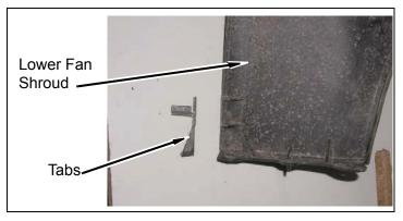
c. Cut lower fan shroud off a long marked corner.
