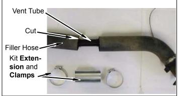
d. Install kit **extension**, **fuel filler** in filler hose with two kit **clamps** (#36).
