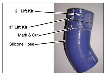
c. Install silicone elbow on intercooler inlet and intercooler piping with two clamps.
