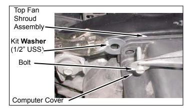
g. Install top fan shroud on bottom fan shroud with four pop-ups. Check fan to shroud clearance. Ensure gap is the same all around shroud.
