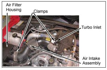
b. Install air baffle and air intake assembly on engine with clamp and torx bolt
