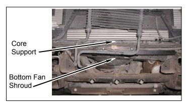
e. Install top fan shroud assembly, computer, and computer cover on core support with four bolts. Do not tighten.
