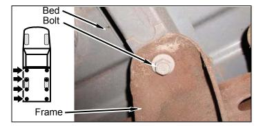
b. Remove four bed bolts from frame passenger side.
