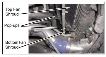
h. Using kit brackets, lower fan shroud support as a template, mark lower fan shroud hole locations as shown. Remove four pop-ups from upper fan shroud and lower fan shroud. Remove lower fan shroud from vehicle.
