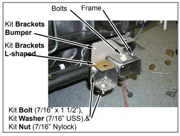
d. 2" kit: Install two kit brackets bumper and two kit brackets C-shaped on frame with two stock bolts, two kit bolts (7/16" x 1 1/2"), four kit washers (7/16" USS), and two kit nuts (7/16" nylock). Do not tighten.
