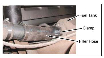
f. Install vent tube in clamp.
