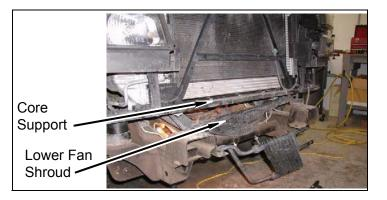
b. Trim tabs from edges of lower fan shroud as shown.
