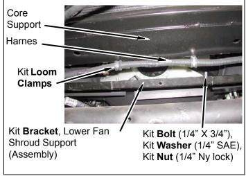
d. Position bottom fan shroud in vehicle and rest below lower fan shroud mounting brackets.
