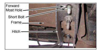
q. Install kit brackets (rear bumper) and hitch on frame with two long bolts, two kit washers (1-1/2 x 2-1/2 rectangular), two kit washers (14mm), into two kit nuts (14mm nylock).
