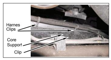
b. Position two kit **loom clamps** on harness.
