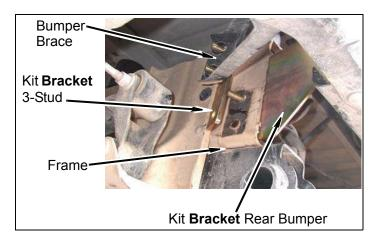
g. **3" kit passenger side:** Install kit **bracket** (3-stud) on outer bumper brace with two kit **washers** (1/2" USS), and two kit **nuts** (1/2" nylock), on two studs as shown. Do not tighten
