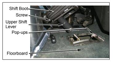
b. Mark upper shift lever and shift lever input shaft to maintain alignment during installation.
