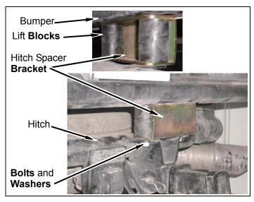
Install hitch on frame with two short bolts and nuts. Use forward most hole in hitch.
