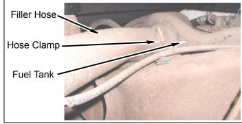
c. Carefully cut filler hose where shown. ENSURE YOU DO NOT CUT THROUGH PLASTIC VENT TUBE INSIDE FILLER HOSE.
