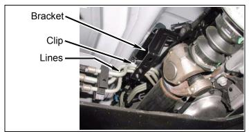
b. Remove two nuts and bracket from transfer case. <u>Bracket is not reused.</u> Install two nuts and tighten.
