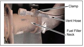
Remove hose clamp and filler hose from fuel tank. Ground wire can be left attached to fuel filler neck.
