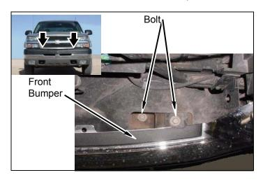
d. Remove six bolts, and two tow hooks from frame.
