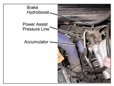
Loosen power assist pressure line fitting at brake hydroboost housing and position power assist pressure line along side of accumulator as shown. f. Tighten power assist pressure line fitting at brake hydroboost housing.
