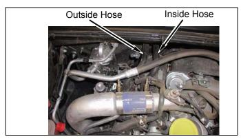
Install kit heater hose 5/8" x 14" and two kit hose clamps #28, on fire wall and heater piping.
