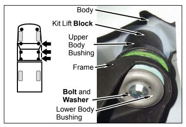
d. Lower cab onto kit lift blocks.
