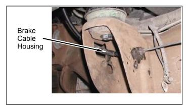
d. Install two ground wires on frame mounting pad with bolt. Connect front and rear brake cables. Remove clamps from rear cable.
