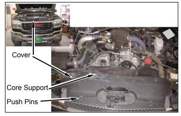
b. Remove bolt, six clips, and grille from core support. Some GMC models may have extra clips.
