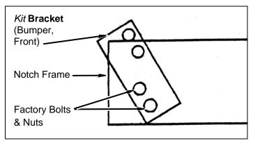
b. Cut two front factory bumper brackets for clearance with frame and factory bumper hardware as shown.
