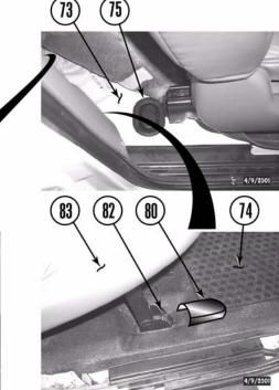
e. Install two rubber caps (75) in front of cab floor (73).
