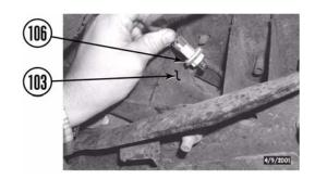
h. If removed, connect trailer hitch connector (105) on rear bumper (103).
