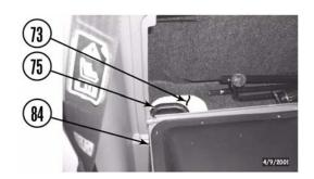
b. Install two rubber caps (75) in middle of cab floor (73).
