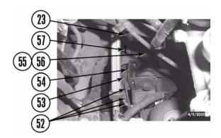
d. If possible, install clip (51) on three ABS lines (52).
