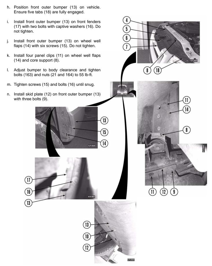
o. Install radiator shroud (6) on grille (7) and core support (8) with two bolts (4) and four screws (5).
