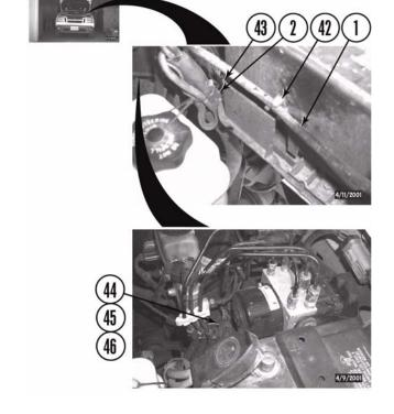
Bend bracket (47) up to release positive cable (2).
