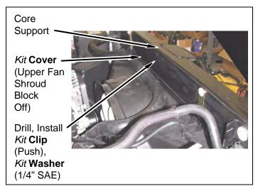
w. Check fan to fan shroud clearance. Ensure gap is uniform around shroud and tighten all nuts and bolts.
