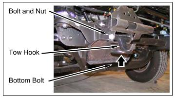
4. Remove bolts and tow hook covers from frame rails.
