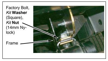
f. Install kit bracket (trailer hitch) to rear bumper and trailer hitch (if equipped) with two kit bolts (14mm x 110mm) and two kit washers (14mm). DO NOT TIGHTEN.
