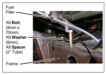
b. Install fuel filler to body with three factory bolts.
