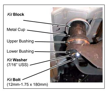
e. Install lower bushing, *kit* **bolt** (12mm-1.75 x 180mm) and *kit* **washer** (7/16" USS) on front core support cab mount. Use factory front core support cab mount nut. DO NOT TIGHTEN.
