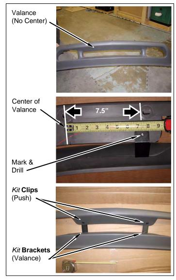
f. If necessary, mark and trim two *kit* **covers** (valance) with dull finish facing outward. Trim lines to match front bumper curve.
