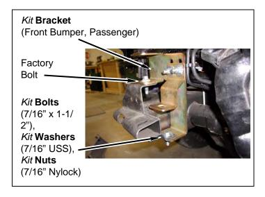
c. Install kit bracket (front bumper, inner passenger) to kit bracket (front bumper, passenger) with two kit bolts (7/16" x 1-1/2"), four kit washers (7/16" USS) and two kit nuts (7/16" Nylock). DO NOT TIGHTEN.
