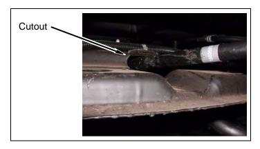
b. Install kit bracket (rear bumper, passenger) to rear bumper with factory hardware, two kit bolts (7/16" x 1-1/2"), four kit washers (7/16" USS) and two kit nuts (7/16" Nylock). DO NOT TIGHTEN.
