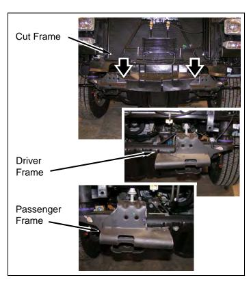
b. Install kit bracket (front bumper, passenger) on frame with factory bolt, kit bolt (7/16" x 1-1/2"), two kit washers (7/16" USS) and kit nut (7/16" Nylock). Apply a few drops of kit Loctite® to factory front bumper bolt. DO NOT TIGHTEN.
