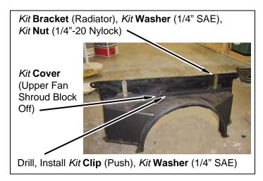
t. Install upper fan shroud assembly on core support, radiator and lower fan shroud with four bolts. Ensure kit cover (upper fan shroud block off) is placed in between core support and radiator.
