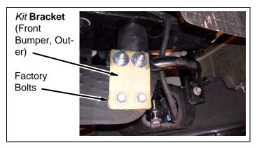
Install front outer bracket to kit bracket (front bumper, outer) with two kit bolts (7/16" x 1-1/2") four kit washers (7/16" USS) and two kit nuts (7/16" Nylock). DO NOT TIGHTEN.
