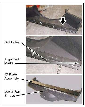
j. Trim locking tabs and marked edges from driver and passenger fan shroud as shown.
