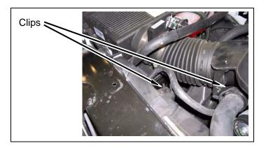
c. Tighten engine air intake hose clamps.
