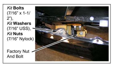
Install kit bracket (front bumper, outer) onto passenger side frame with factory bolts. Apply a few drops of kit Loctite® to threads of factory bolt.
