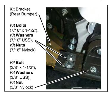
e. Install rear bumper to trailer hitch (if equipped) with two factory bolts, two kit washers (square) and two kit nuts (14mm Nylock). DO NOT TIGTHEN.
