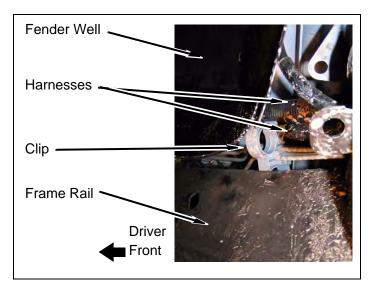
b. Remove harness clips from frame rail. Remove bolts and ground straps from frame.
