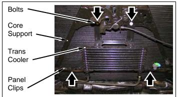
b. Remove cooler lines from core support clip.
