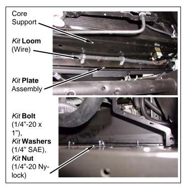
n. Install lower fan shroud on *kit* **plate** assembly with three *kit* **bolts** (1/4"-20 x 1"), six *kit* **washers** (1/4" SAE), three *kit* **nuts** (1/4" nylock) and two *kit* **clips** (push).
