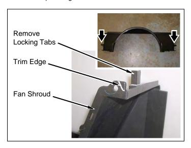
k. Using lower fan shroud as a template, mark upper fan shroud. Trim marked edges from upper fan shroud to coincide with lower fan shroud as shown.
