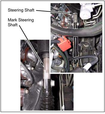
c. Remove bolt, nut and upper steering shaft from lower steering shaft.
