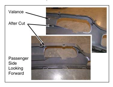
e. **GMC** models without blocked center: Position two *kit* brackets (valance) on lower valance 7.5" from center. Mark and drill four 1/4" holes in lower valance. Install two *kit* brackets (valance) with four *kit* clips (push).
