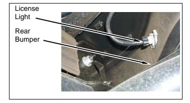
c. 2000-2004 models: Remove three wire harnesses and clips from rear bumper.
