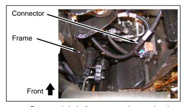
e. Remove six bolts from two rear bumper brackets and frame.
