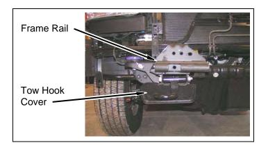
5. Remove bolts and lower guard from core support and frame.
