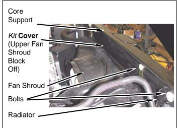
u. Attach upper fan shroud to lower fan shroud with four pop-ups on sides of fan shroud.
