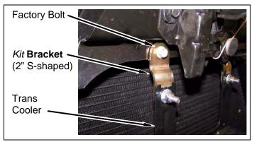
c. Install transmission cooler on two kit brackets (2" S-shaped) with kit washer (1/4" SAE) and kit nut (1/4"-20 Nylock). DO NOT TIGHTEN.
