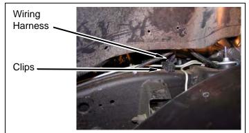
c. Install wire clips to body and frame rail along passenger side, if possible.
