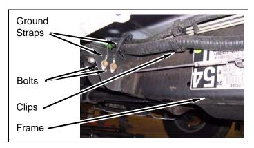
c. Remove wire clips from body and frame rail along passenger side.
