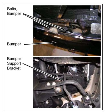
3. Remove bolts and tow hooks from frame rails.
