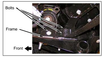
f. If equipped with a trailer hitch, remove four bolts from hitch, rear bumper and frame.
