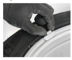
Before installation, the weight matching the rim shape is selected. The build of the rim is used for differentiation. Before installation to the rim, apply the weight to check its fit.
