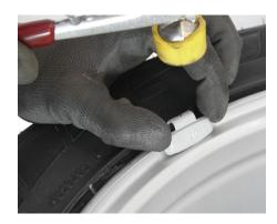
Place the weight at the correct location of the imbalance. Before you knock on the weight with a hammer, make sure that the clip touches the rim flange. The actual body of the weight should not touch the rim.
