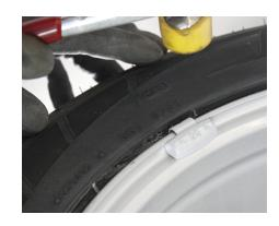
After correctly aligning the weight, it is knocked on with the corresponding installation hammer. Do not use more than two strong hits for installation. Note: Increasing the impact number can damage the weight coating.
