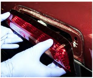
Using the T20 Torx Driver, remove the two screws holding the brake light housing in place and pull the brake light away from the cab.
