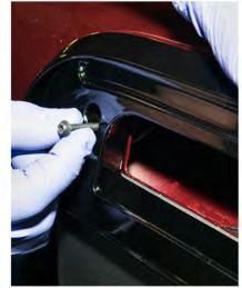
Route the cable into the cab following the brake light harness. Seat the adapter as shown. Use the two OEM T20 screws to secure the antenna adapter to the cab using the factory holes.
