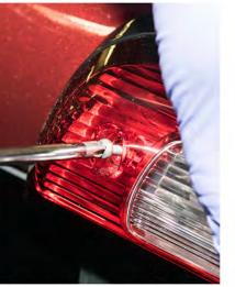
Tighten the screws on the antenna mount clamp until they are snug. Reconnect the wiring harness and guide the pin from the brake light housing into the machined holes of the antenna mount. Use the supplied screws to secure the OEM brake light housing to the antenna adapter.
