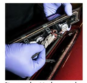
Disconnect the wiring harness and set the brake light housing aside.
