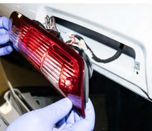
Using the Phillips Head Screwdriver, remove the two screws holding the brake light housing in place and pull the brake light away from the cab.
