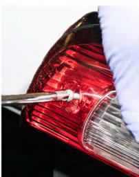
Tighten the screws on the antenna mount clamp until they are snug. Reconnect the wiring harness and guide the brake light housing to line up with the machined holes of the antenna mount. Use the supplied screws to secure the OEM brake light housing to the antenna adapter.
