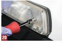
**Fig. 17-18** Attach the bulbs and power connector in the reverse manner as removal. **Fig. 19** Route the harness and back of the light housing to avoid interference with the antenna cable, as it is positioned back in place. **Fig. 20** Re-install the light housing utilizing the factory hardware. With the 3rd Brake Light Antenna Adapter installed, attach desired compatible antenna with NMO standard threaded antenna connector and fasten the PL-259 male UHF connector to preferred 2-way radio.
