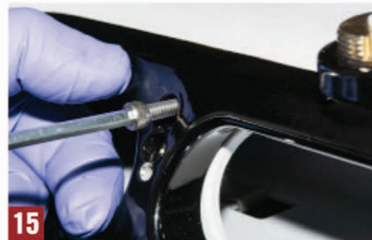
Fig. 8 Route the antenna cable into the cab - follow the brake light harness. From inside the cab, access the cable and route to final desired location. Fig. 9-12 To attach the antenna adapter, align and attach the adapter utilizing the four (4) factory mounting holes and the provided phillips pan head screws. Fig. 13-15 Keep the adapter secured in place. Using the adapter's two (2) top center holes as a guide, drill through the truck body with a 3/16" bit. Next, feed the support bracket through the middle hole of the adapter. Slide the support bracket behind the adapter and the truck body then, match up the support bracket's holes with the ones you just drilled. Use the provided socket head cap screws to secure the support bracket in place.
