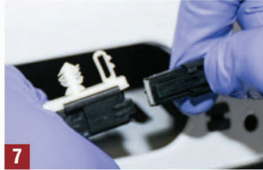
Fig. 2-3 Using a 9/32"(7mm) nut driver, remove the four (4) screws holding the housing in place and pull away from the cab. Fig. 4-7 Disconnect the light housing at the pigtail connector - not at the light. Access the connector by pushing down on the clips and pulling through the opening on the right. Disconnect by pressing down on the retaining clip, then slide away from each other. Place the removed housing in a safe location to be re-installed later.
