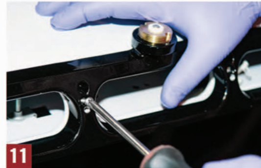
Fig. 8 Route the antenna cable into the cab - follow the brake light harness. From inside the cab, access the cable and route to final desired location. Fig. 9-12 To attach the antenna adapter, align and attach the adapter utilizing the four (4) factory mounting holes and the provided phillips pan head screws. Fig. 13-15 Keep the adapter secured in place. Using the adapter's two (2) top center holes as a guide, drill through the truck body with a 3/16" bit. Next, feed the support bracket through the middle hole of the adapter. Slide the support bracket behind the adapter and the truck body then, match up the support bracket's holes with the ones you just drilled. Use the provided socket head cap screws to secure the support bracket in place.
