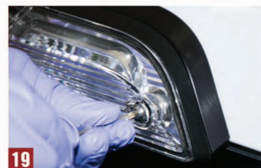
Fig. 16 Re-connect the light housing in the reverse manner as removal. With the power harness attached, route back through the opening and with the clips aligned with the small openings push up to attach back in place. Fig. 17-19 Re-install the light housing utilizing the provided longer button head cap screws for the middle two (2) holes and the shorter button head cap screws for the outer two (2) holes. With the 3rd Brake Light Antenna Adapter installed, attach desired compatible antenna with NMO standard threaded antenna connector and fasten the PL-259 male UHF connector to preferred 2-way radio.
