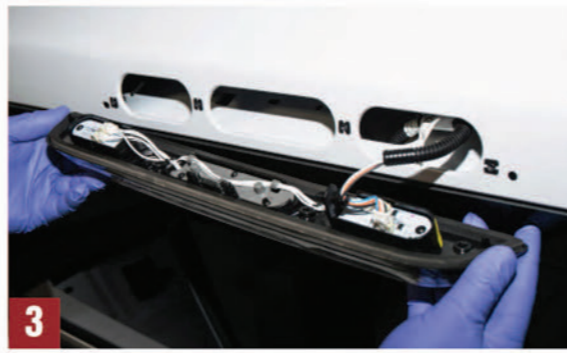
Fig. 2-3 Using a 9/32"(7mm) nut driver, remove the four (4) screws holding the housing in place and pull away from the cab. Fig. 4-7 Disconnect the light housing at the pigtail connector - not at the light. Access the connector by pushing down on the clips and pulling through the opening on the right. Disconnect by pressing down on the retaining clip, then slide away from each other. Place the removed housing in a safe location to be re-installed later.
