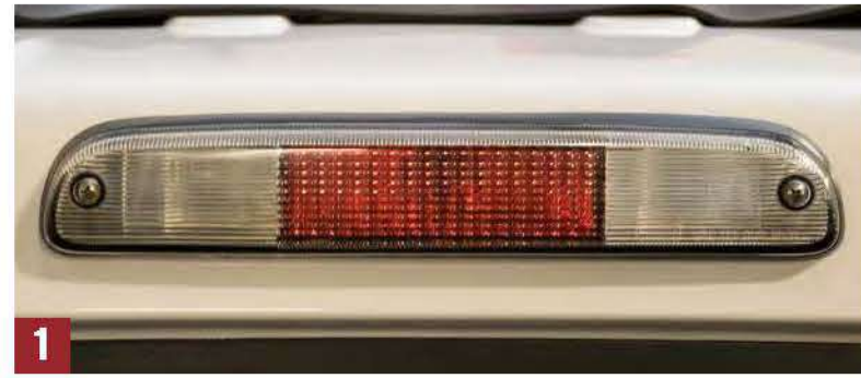
Fig. 2-3 Using a phillips screwdriver, remove the two (2) screws holding the light housing in place and pull away from the cab. Fig. 4-5 Disconnect the light housing by rotating the bulbs counter-clockwise, then pull straight out to remove from the light housing. Next, release the entire harness from anchor point on the housing by pulling back on the retaining clip below the power connectors, then slide away from the housing. NOTE: The power connectors remain connected to each other. Place the removed light housing in a safe location to be re-installed later.
