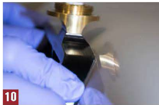
Fig. 6 Route the antenna cable into the cab following the brake light harness. From inside the cab, access the cable and route to final desired location. Fig. 7 Route the bulbs and harness through the middle of the antenna adapter. Fig. 8-10 To attach the antenna adapter, hook the top of the cab opening between the support bracket and antenna adapter, then rotate the bottom of the adapter into position. Fig. 11-12 Using the factory installation screws, temporarily attach the adapter utilizing the factory mounting holes. Using the 5/32" allen wrench, tighten the two (2) support screws to sandwich the cab between the bracket and the adapter. Fig. 13-14 Remove the factory installation screws.
