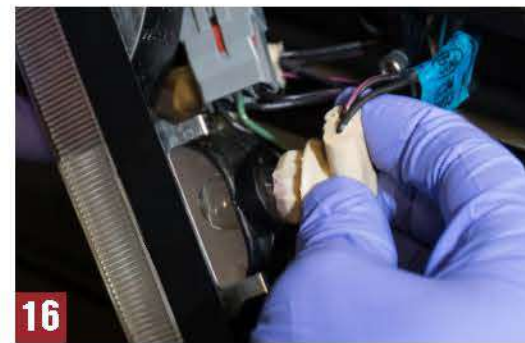
Fig. 16 Route passenger side cab light bulb behind the support bracket and back through the antenna adapter opening. Fig. 17-18 Attach the bulbs to the light housing starting with the passenger side, then middle brake light bulb and finally the driver side. NOTE: The power connectors WILL NOT be re-attached to the anchor point on the light housing. Route the harness and back of the light housing to avoid interference with the antenna cable as it is positioned back in place. Fig. 19 Re-install the light housing utilizing the provided hardware. With the 3rd Brake Light Antenna Adapter installed, attach desired compatible antenna with NMO standard threaded antenna connector and fasten the PL-259 male UHF connector to preferred 2-way radio.
