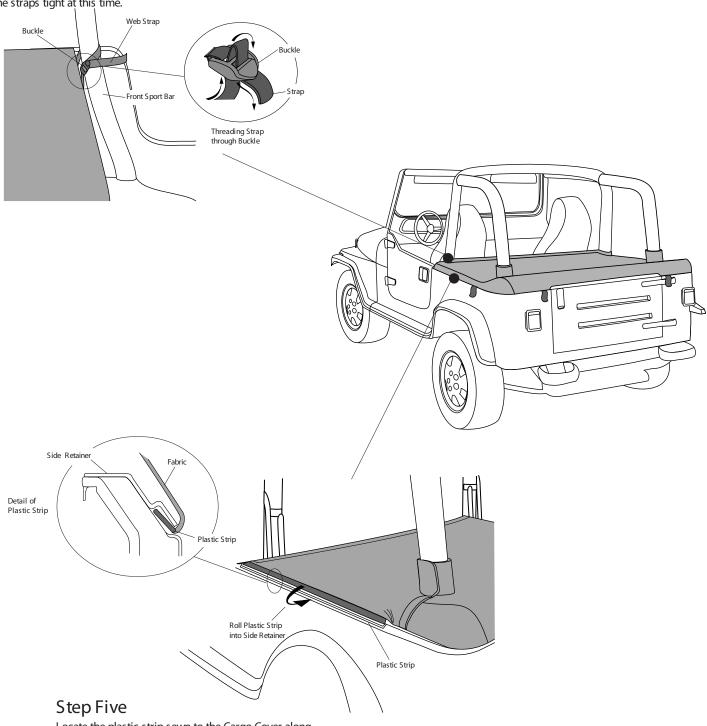
Locate the plastic strip sewn to the Cargo Cover along each side of the vehicle. Start at one end on each side and roll the plastic strip into the Side Retainers.
