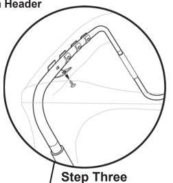
Use a phillips screwdriver to remove the four (4) screws that attach the flaps in the top to the Rear Bow. Allow the bow to drop onto the tailgate **Set the screws aside to be reused later.**
