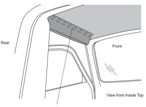
Wrap flap around door frame and fasten hook and loop
