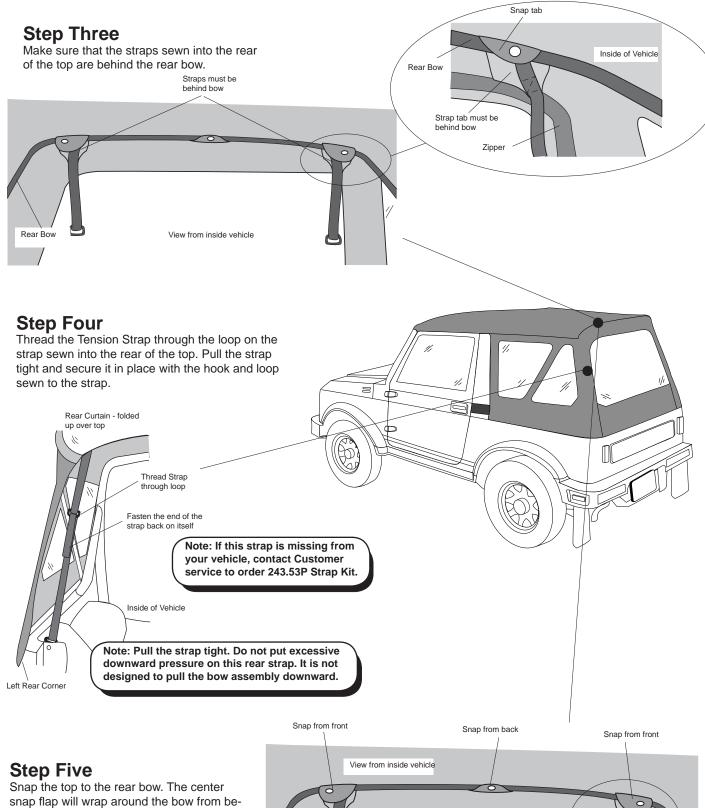
Snap the top to the rear bow. The center snap flap will wrap around the bow from behind and the two outer snap flaps will wrap around the bow from the front.
