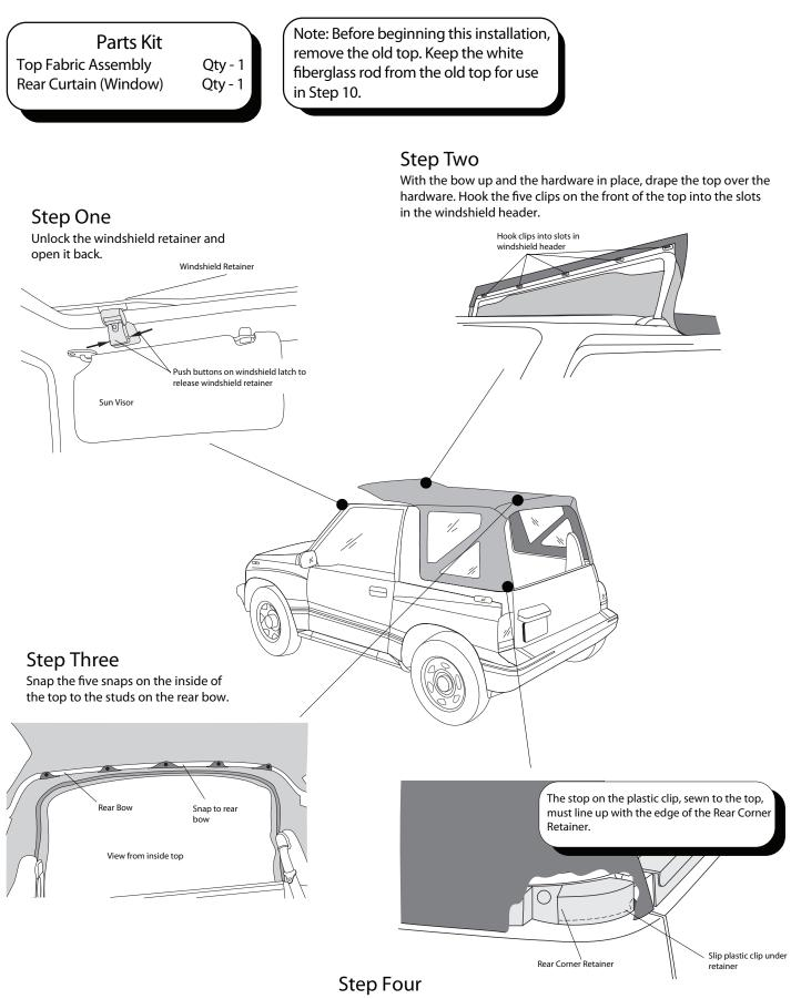
Locate the plastic clips sewn into each rear corner of the top. Pull down and back on the top fabric and slip them into the space under the plastic corner retainer attached to the vehicle. The stop on the inside edge of the plastic clip on the top should line up with the inside edge of the retainer.
