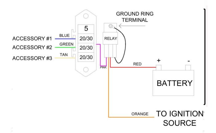
E: POPULATE THE FUSE BLOCK WITH THE APPROPRIATELY RATED FUSE FOR EACH CIRCUIT. KEEP IN MIND THE RELAY IS DESIGNED TO HANDLE 70 AMPS OF CONTINUOUS CURRENT. DO NOT ATTEMPT TO DRAW MORE THAN 70 AMPS OF CURRENT THROUGH THIS CIRKIT BOSS KIT. DOING SO WILL CAUSE PREMATURE FAILURE OF THE RELAY.
