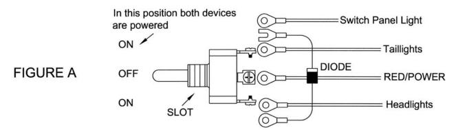
NOTE: The diode is to be used when wanting to operate two devices and have them both powered in one of the on positions.
