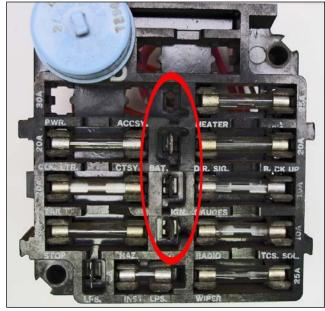
the key is in the ACCESSORY position, plug the connector into the ACC port. For the windows to only work in the ON position, plug the connector into the IGN port.
