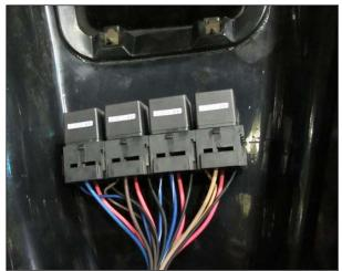
At this point the new harness is completely installed. Before components like the driver side seat, door sill and kick panels are installed you should test that everything is working.
