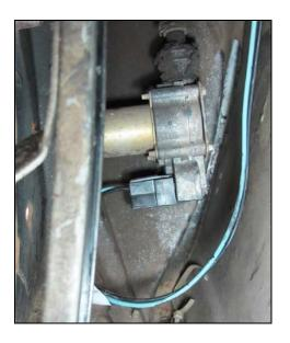
If you find that your actuator(s) are faulty or simply missing, they can be replaced by using ACDelco part # 22020256
