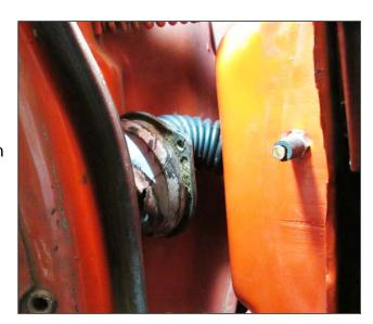
Once the door grommet is installed, go to the kick panel area where the door harness enters into the inside of the vehicle. Locate the grommet and pull it through and seat the grommet into the small hole on the interior. All three seating ridges can be seen on the door grommet shown on page 2.
