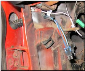
Pull the grommet through the hole in the door, and feed it into the inside of the car until the grommet matching the hole in the body is through the door, seen on page 2. You will seat the grommet into the car body (door jamb). A flat head screw driver will make it easier to get the grommet seated.
