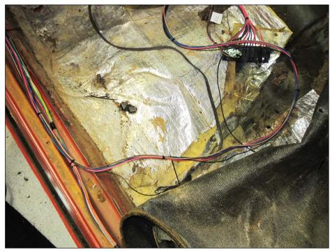
Route the wires through the notch to the center of the car.
