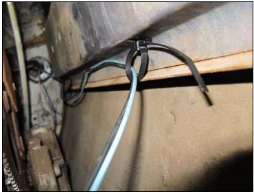
With the wires now routed down the length of the door, connection to the lock actuator can take place. In order to plug the connector into the actuator, the tab on the connector must be pressed down while the connector is being plugged into the actuator. This will raise the locking tab to allow it to fit over the connection point. Once connected go back and tighten any zip ties that may have been installed in the channel.
