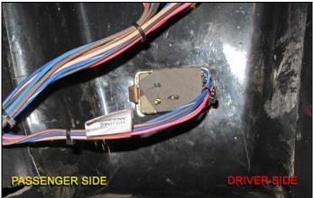
If a replacement window switch is needed GM #1725092 can be used to help you locate one new or reproduced from online sources/auctions or numerous fbody part vendors.
