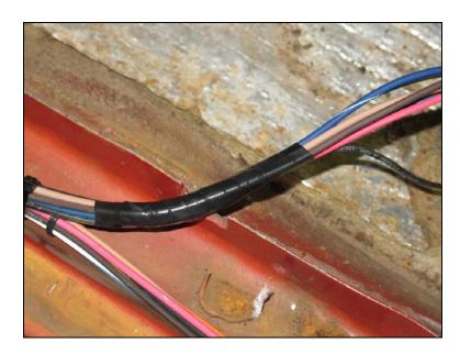
Route the window switch connector to the console mounted window switch and connect. To ensure the driver side switch operates the driver side window, the wires going into the connector must be on the driver side of the console.
