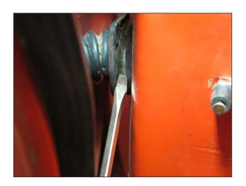
You will next seat the big end of the grommet into the door. This is done by pulling the entire grommet through the hole and then reinserting from the jamb side back into the door, as shown below.
