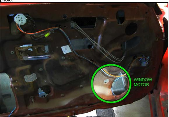
Route the Window Motor connector to the window motor and connect. This connector will only plug in one way. Be sure to route the wires away from the regulator and window track to avoid any interference with the operation of the window.
