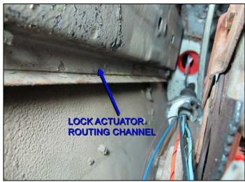
Route the two wires down this channel towards the rear of the door. There may be factory clips along the top of this channel for you to attach the harness to.
