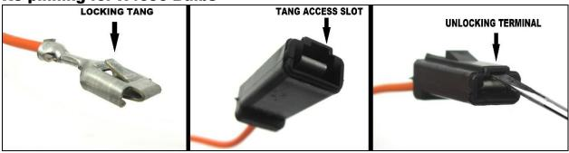
Notice the locking tang that holds the terminal in the connector. Locate the tang access slot on the terminal end of the connector. The connector in the photo is just an example and not a connector found on the 30815 harness. Push a paper clip, stiff wire, or a small flat head screwdriver into the slot to depress the locking tang on the terminal.
