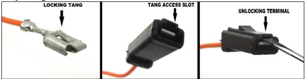
Notice the locking tang that holds the terminal in the connector. Locate the tang access slot on the terminal end of the connector. The connector in the photo is just an example and not a connector found on the 30814 harness. Push a paper clip, stiff wire, or a small flat head screwdriver into the slot to depress the locking tang on the terminal.
