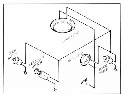
**<u>NOTE</u>**: BY ATTACHING THE BLACK WIRES OF BOTH LIGHTS TOGETHER, AND THEN TO THE JAMB AND/OR LIGHT SWITCH, BOTH LIGHTS WILL COME ON AT THE SAME TIME.
