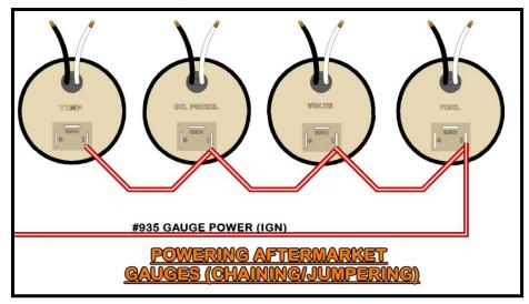
Grounds need to be supplied to the gauge lights and any ground tab on the gauges. The installer needs to run their own ground circuit for gauge connections. To make these ground connections you can splice from the installer provided ground wires to all the gauges or chain/jumper it all together. Both methods can be seen in the following two drawings:
