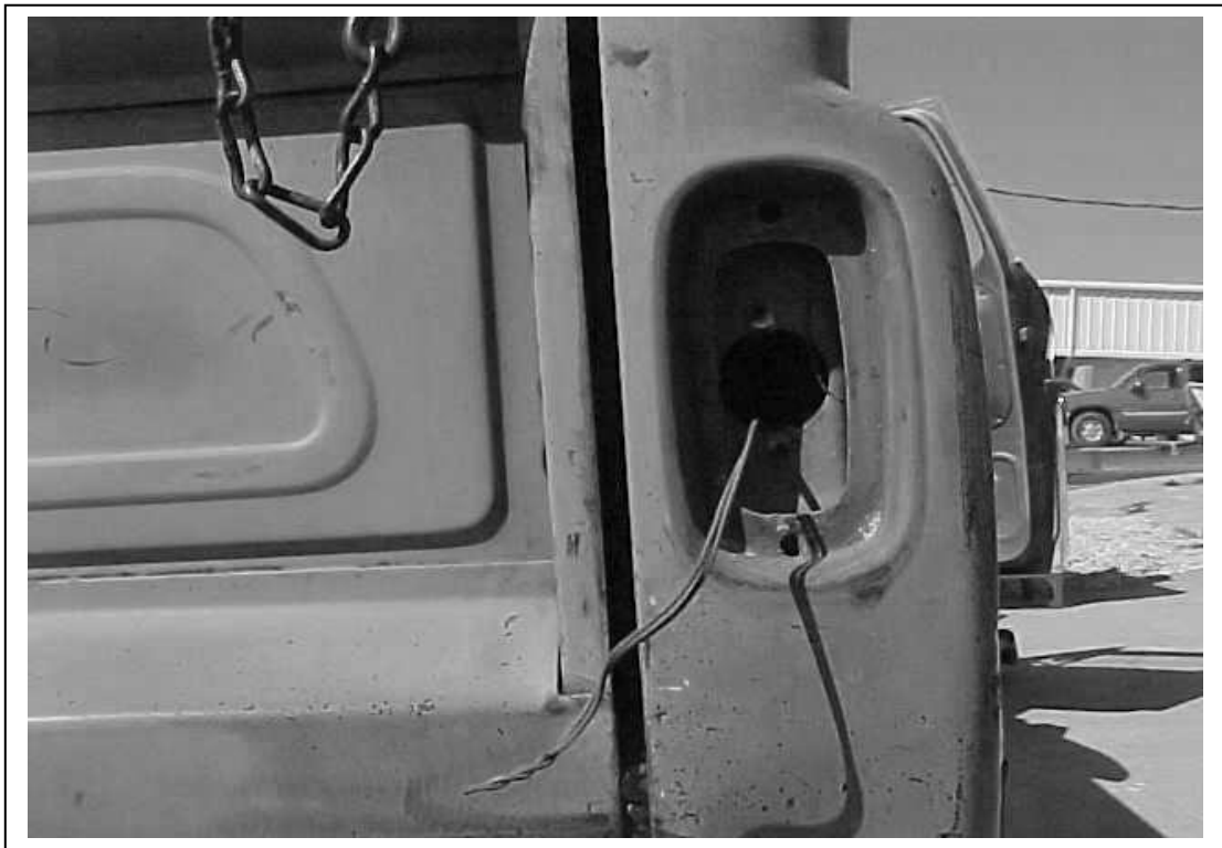
Figure 7.14 Tail Lights removed, wire ready to measure, cut, splice and re-install
