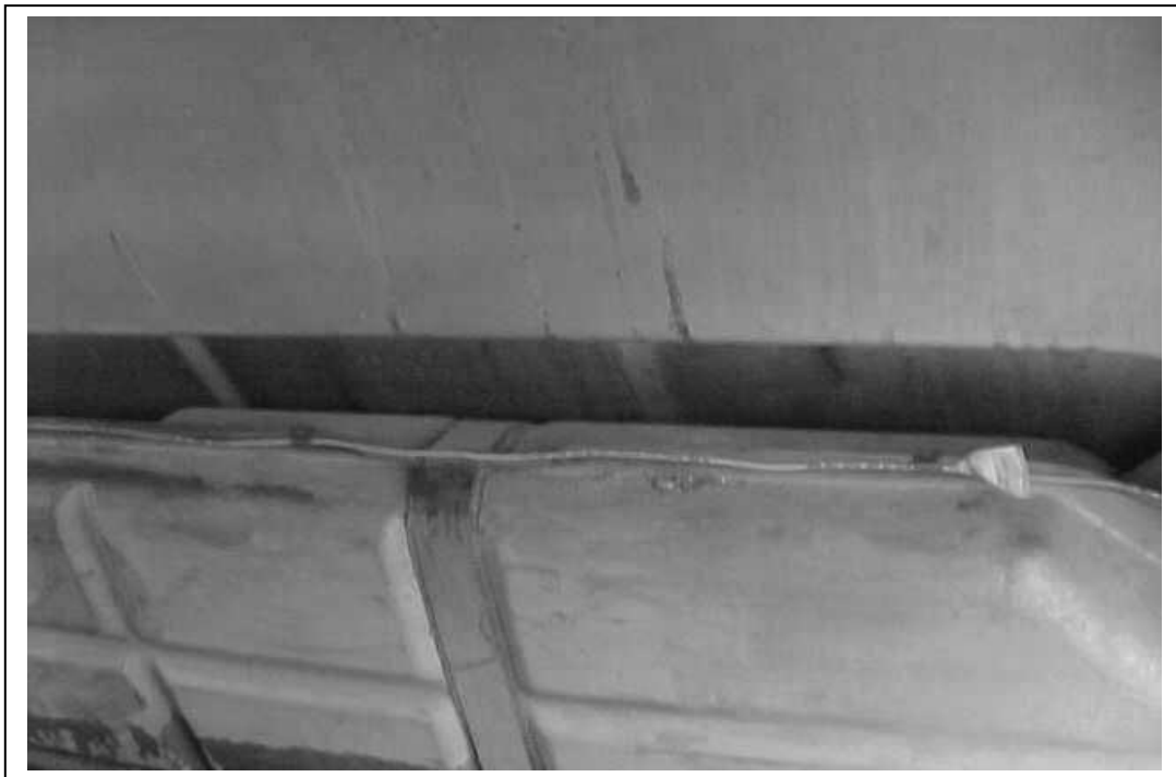
Figure 6.8 Cab mounted fuel tank, has mounting clips on the seam of the tank.
