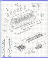
Volvo / Renault Engine Components 2015 Cylinder Head - Volvo D11 / D13
