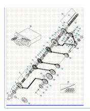
**Web Electronic** Main Case Components - Fuller Transmission
