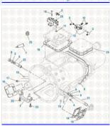
**Drive Train 2016** Compound and Main Case Assembly - T313L and T318L
