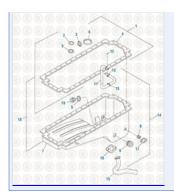
**Cummins Engine 2017** Oil Pan and Components - N14 Series
