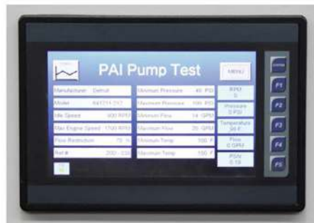
Oil Pump Testing System Control Panel
