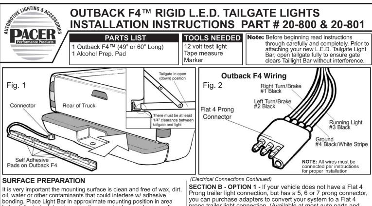
below tailgate to determine mounting area to clean and prepare for installation. Take the Alcohol Preparation Pad supplied and clean mounting surfaces thoroughly.
