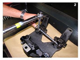
Failure to do so may cause interference between the spring and intake valve. Use a hand torque wrench (not a pneumatic or impact) to tighten the button head screw to 180 lb\*in.
