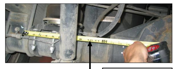
This vehicle is shown with the breather located 10" from leaf spring pack and does not require the 10136.
