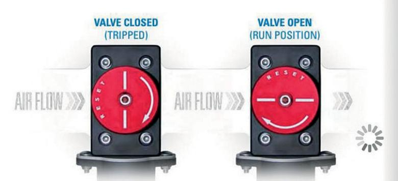
CAUTION: The #1 failure mode of any valve in the market is seizing due to lack of use. As this is a safety device, it is imperative that you employ safety activation testing at a minimum of once per month.
