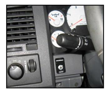
2 Remove the driver side knee panel to gain access to the base of the steering column.
