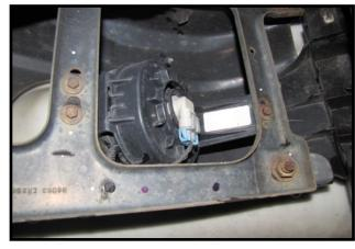
Route the Pacbrake harness forward and down to the compressor, connect the mating Metri-Pac connector of the compressor assembly to the harness. Continue routing the harness toward the air tank, connect the mating Metri-Pac connector of the harness to the pressure switch.
