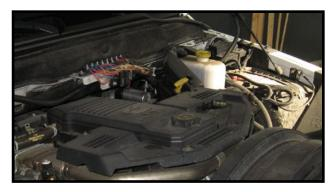
Install the 1/4"NPT-1/4" push on barbed hose fitting onto the plastic filter housing. Locate the Blue nylon hose and connect one end to the barbed fitting on the intake filte. Install the compressor air intake filter into the hole located in the radiator support bracket behind the driver side headlight as shown in the photo. Or any cool dry location. Route this line down to the driver side rear of the bumper.
