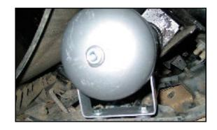
Connect the Black nylon airline to the remaining fitting at the compressor. Route it to the top of the air tank. Cut the airline to length with a sharp razor knife. Connect the ¼" airline to either fitting in the tank. Secure the airline away from moving parts and heat sources using the tie straps provided.
