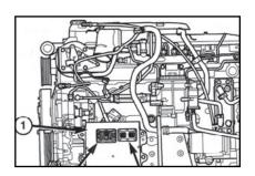
27 At the 50 pin (rear) connector, locate pin #42 and remove the sealing plug. Be careful not to push it in Once the sealing plug is removed, insert the black wire with the special ECM pin from the compressor harness into cavity #42 Push in until seated Gently pull o the wire to ensure the pin is locked in place.
