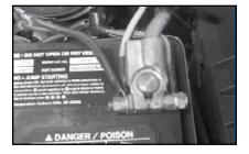
Connect the black wire with the eye terminal to the negative battery terminal or a good chassis ground.
