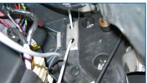
Locate the diagnostic connector under the dash on the drivers side. Remove the two screws fastening it to the dash. Connect the male/female plugs of the Pacbrake harness to the factory diagnostic connector, secure the Pacbrake connector to the lower dash panel using the original screws. Secure the two connectors with a tie strap.
