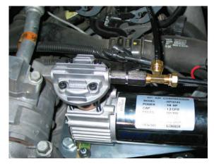
Locate the black nylon airline connected to the air tank in step 5. Route the airline away from moving components and heat sources to the air compressor. Secure with the tie straps provided. Connect the airline to the "tee" fitting at the air compressor.
