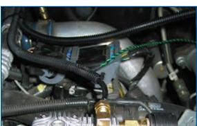
Locate the air cylinder breather hose (blue) in the engine compartment installed in step 4. This hose connects to the air compressor inlet filter with the "T" fitting provided. Connect the filter, the air compressor intake and the cylinder breather hose as shown. The filter housing is installed into the hole below the radiator in the support bracket. Secure the breather hose with the tie straps provided.
