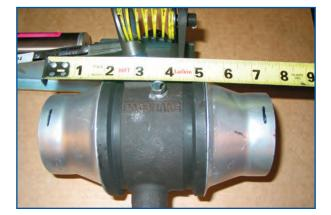
Select a location in the exhaust system that has sufficient clearance for installation and servicing of the exhaust brake. This location should be as close to the turbocharger as possible and away from dirt and road spray. Transfer the brake/adapter measurement, attained in step 2, to this location and mark the exhaust pipe. Remove the exhaust pipe and cut out the pre-marked section.
