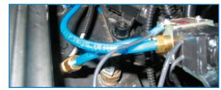
7 Using the short hose with breather vent installed, connect to port #3 of the solenoid valve. Route this breather to a location free from water and dirt.
