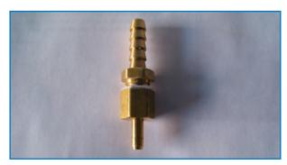
Locate one of the two brass fittings assembled in step 5. Connect the white vacuum line removed in step 5 to the barbed end. Locate the short blue nylon line supplied and connect to the other end of the fitting. Connect the blue nylon line to the Pacbrake solenoid port #2.
