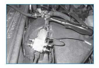
Locate transfer case vacuum lines adjacent to transmission <u>above starter on driver's side</u> of vehicle (green line = vacuum vent / white line = vacuum source)
