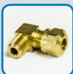
C11796 MALE PIPE 90° ELBOW Material: Brass Fitting End A: ¼" OD Tube Nylon Fitting End B: ⅛" (-2) NPT Male DOT
