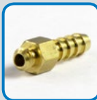
C10686 MALE PIPE CONNECTOR Material: Brass Fitting End A: 1/8" ID Tube Fitting End B: 10/32" UNF Male
