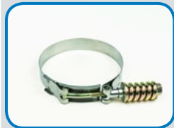
C3977 SPRING LOADED Min: 3.875" [98.4 mm] Max: 4.188" [106.4 mm] Band width: 0.75" [19.1 mm] SAE: 96
