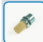
C10774 POROUS BRONZE AIR SILENCER Material: Bronze/Steel Fitting End A: ⅜" (-2) NPTF Male Max Rated: 5 SCFM @ 90 psi
