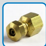
HP1151 FEMALE PIPE CONNECTOR Material: Brass Fitting End A: ¼" OD Tube Nylon Fitting End B: ¼" (-4) NPT Female DOT
