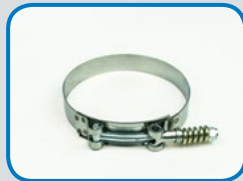
C3876 SPRING LOADED Min: 4.063" [103.2 mm] Max: 4.375" [111.1 mm] Band width: 0.75" [19.1 mm] SAE: 102
