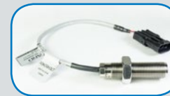
C50033 MAG PICK UP HALL EFFECT SENSOR LENGTH: 2" [50.8mm] THREAD: 5/8 - 18 UNF
