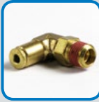
HP1122 MALE PIPE 90° SWIVEL ELBOW Material: Brass Fitting End A: 1/8" OD Tube Fitting End B: 1/8" (-2) NPT Male (Pre-Applied Sealant) NON-DOT
