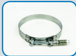
C3879 SPRING LOADED Min: 4.75" [120.7 mm] Max: 5.063" [128.6 mm] Band width: 0.75" [19.1 mm] SAE: 124
