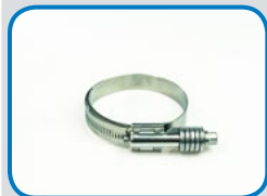
C3976 GEAR CLAMP Min: 2.25" [57.2 mm] Max: 3.125" [79.4 mm] Band width: 0.625" [15.9 mm] SAE: 312
