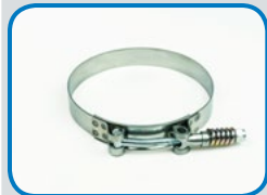
C3878 SPRING LOADED Min: 4.5" [114.3 mm] Max: 4.813" [122.2 mm] Band width: 0.75" [19.1 mm] SAE: 116
