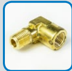
C20092 90° STREET ELBOW Material: Brass Fitting End A: 1/8" (-2) NPT Male Fitting End B: 1/8" (-2) NPT Female
