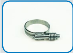
C3975 GEAR CLAMP Min: 1.75" [44.5 mm] Max: 2.625" [66.7 mm] Band width: 0.625" [15.9 mm] SAE: 262
