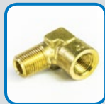
HP1171 90° STREET ELBOW Material: Brass Fitting End A: 1/4" (-4) NPT Male Fitting End B: 1/4" (-4) NPT Female
