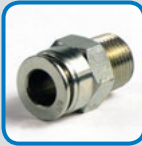
HP1098 MALE PIPE CONNECTOR Material: Nickel Plated Brass Fitting End A: 1/4" OD Tube Fitting End B: 1/8" (-2) NPT Male NON-DOT
