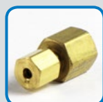
HP1120 FEMALE PIPE CONNECTOR Material: Brass Fitting End A: ⅛" OD Tube Nylon Fitting End B: ⅛" (-2) NPT Female NON-DOT
