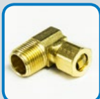
HP1236 MALE PIPE 90° ELBOW Material: Brass Fitting End A: ⅜" OD Tube Brass/ Copper/Aluminum Fitting End B: ⅜" (-6) NPT Male NON-DOT
