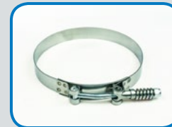
C3880 SPRING LOADED Min: 5.125" [130.2 mm] Max: 5.438" [138.1 mm] Band width: 0.75" [19.1 mm] SAE: 136
