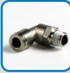
HP1019 MALE PIPE 90° SWIVEL ELBOW Material: Nickel Plated Brass Fitting End A: 1/4" OD Tube Fitting End B: 1/8" (-2) NPT Male (Pre-Applied Sealant) NON-DOT
