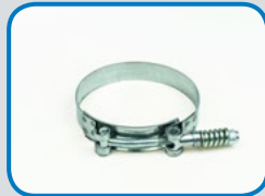
C3874 SPRING LOADED Min: 3.5" [88.9 mm] Max: 3.813" [96.8 mm] Band width: 0.75" [19.1 mm] SAE: 84
