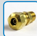
C10570 MALE PIPE CONNECTOR Material: Brass Fitting End A: ¼" OD Tube Nylon Fitting End B: ⅜" (-2) NPT Male DOT
