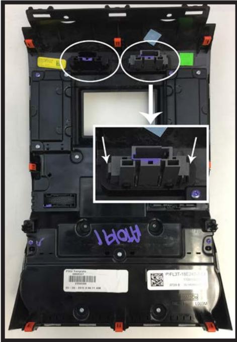
1. Remove hazard and traction control buttons from factory dash panel by pushing in on the release tabs. Set aside for later use.
