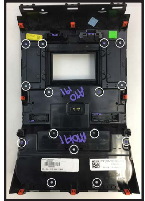
3. Remove (15) T10 22mm screws from factory dash panel. Set (3) aside for later use.
