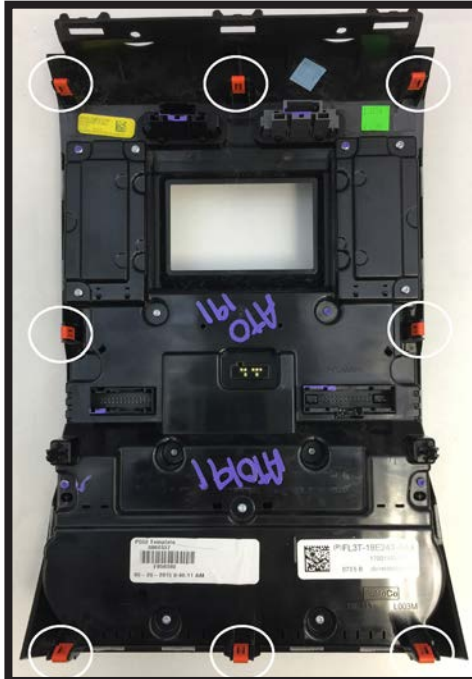
2. Remove (8) orange clips from factory dash panel using a small flathead screwdriver. Set aside for later use.
