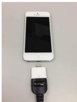
To regain proper control and operation, you must disconnect the (Lightning to 30-pin) adaptor from the GateWay cable.
