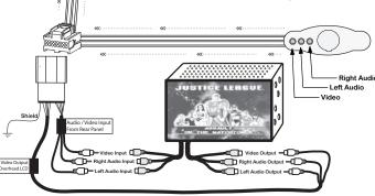
**Note:** This cable is intended for use in conjunction with an OS-4 to retain all safety and convenience systems. The vehicle should be equipped with a Panasonic Overhead LCD and IR system, in which the DVD player was part of the AM/FM/CD receiver. The OS-4 is needed to power the IR headphone system.
