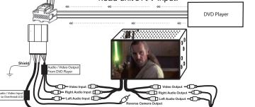
**Note:** This cable is intended for use in conjunction with a C2R-CHY4 (Rev 1.1.4 or higher) to retain all safety and convenience systems. The vehicle should be equipped with a factory Overhead LCD and IR system, in which the DVD player was either part of the AM/FM/CD receiver or a seperate stand alone unit.
