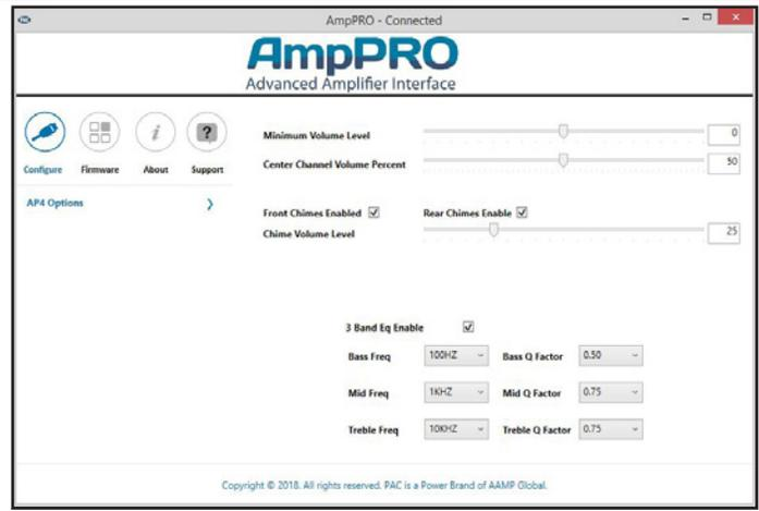
**PLEASE NOTE:** These settings can be adjusted with the module installed in the vehicle, or on the bench. However, it is recommended to make the adjustments with the module installed, and the factory radio on, so that the changes can be heard.
