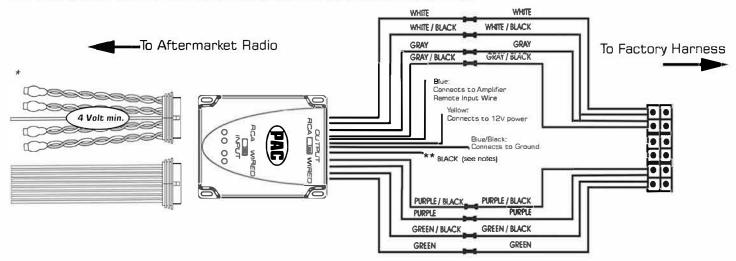
\* Note: 4 volt min. RCA level, if using RCA signal as INPUT to SOEM-4.
