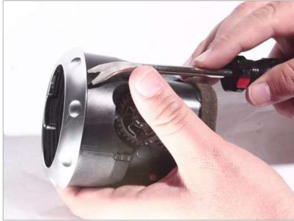
1 Gently pry off aluminum adjuster ring.
