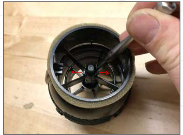
7a Use a screwdriver to spread tabs and release center shaft as shown
