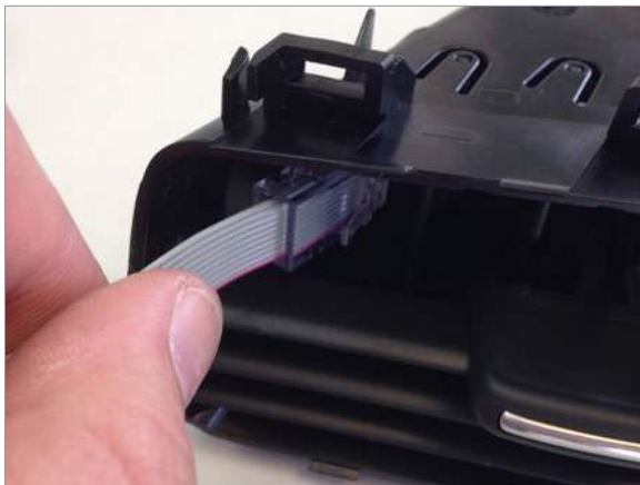
11 Feed the display cable into the vent housing on the far left side of the vent.
