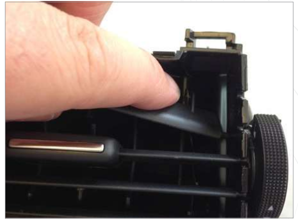
10 With a small flat head screw driver release vent slat from retainer clip as seen here highlighted by finger.
