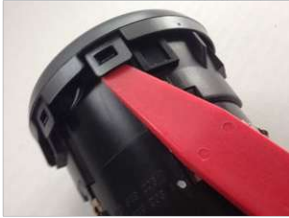
1 Release the clips on connecting the vent facia to the vent housing.
