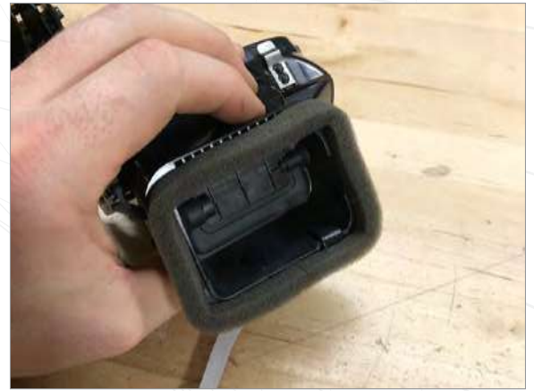
11 Fold ribbon cable around back of vent housing and glue foam back in to place.
