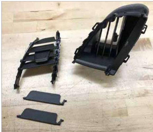
3 Remove bottom two vent slats from assembly.
