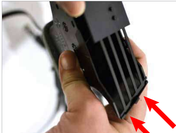
6 Insert the display into the vent tube and secure its aluminum tabs into the 4 slots, 2 on each side. Feed the excess cable out the rear of the vent.
