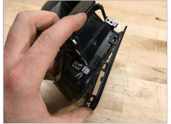
13 Reinstall trim on to vent housing.
