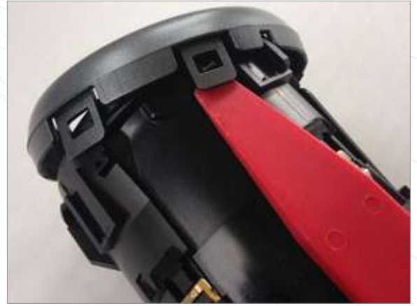
2 Release the final clip connecting vent facia to the vent housing.
