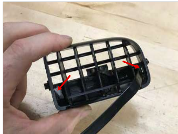
7 Glue display into place by placing glue on both tabs where shown.
