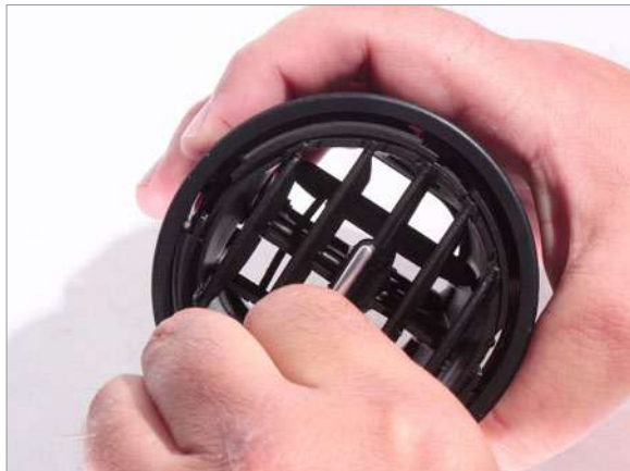
4a Remove slats by loosening slat ends.
