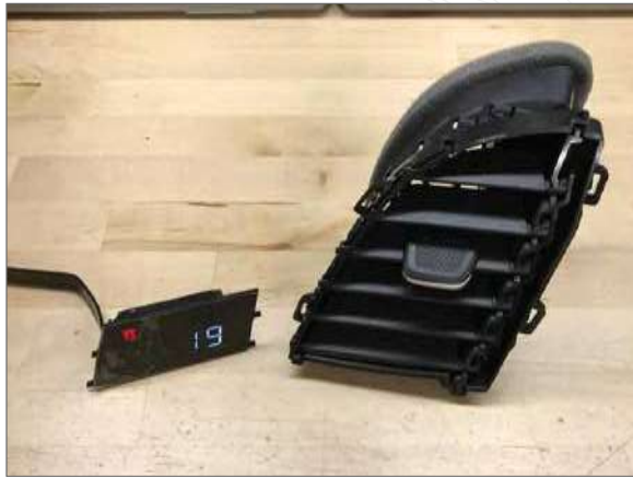
1 Remove vent from vehicle.
