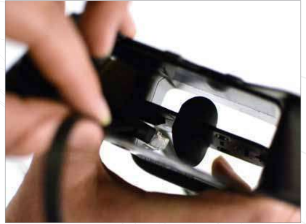
5b The cable is flat as not to interfere with the vent functions and exit through the back of the vent without any cutting.
