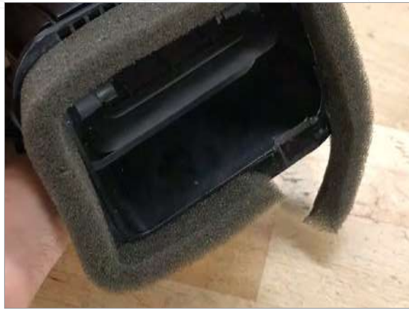
10b Pull foam away from vent as shown.
