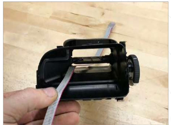
8 Feed cable through vent housing as shown.
