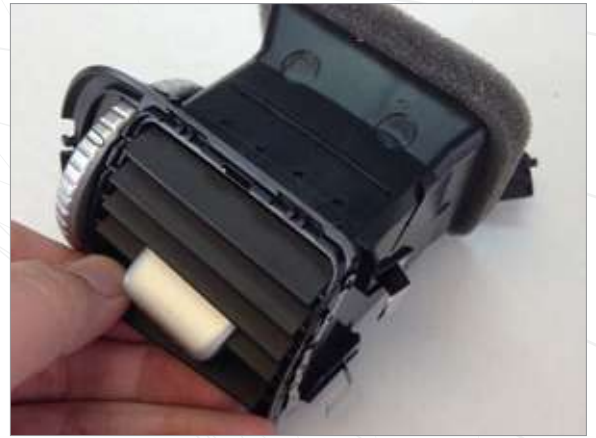
8 You will now be removing the bottom 3 horizontal vent slats. Unclip the slat under the left right control starting at the left most part of the vent housing.
