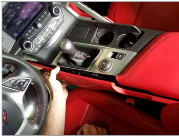
7 Remove console trim and set aside
