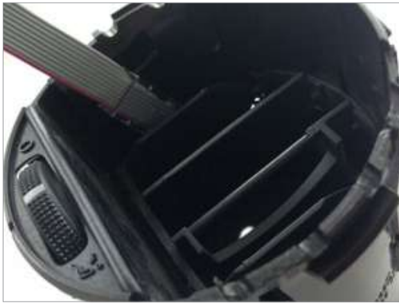
9 Feed display cable in on far left side of vent between the vent wall and the last vertical slat.
