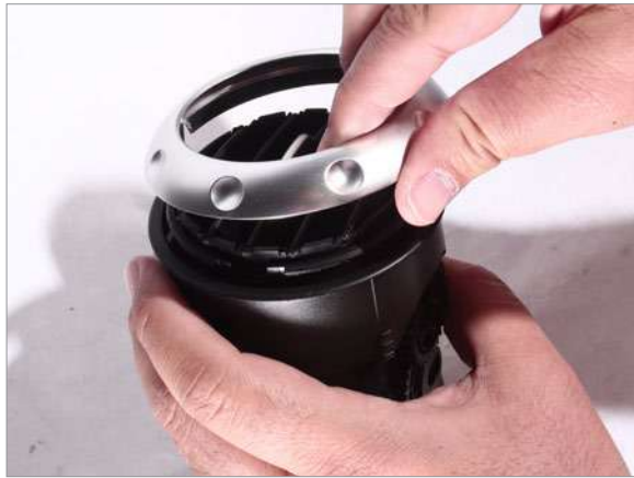
3 Remove trim ring and set aside. Notice that the ring has an indexing notch that you will need to line up when reinstalling.
