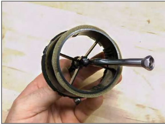
7b Push center shaft toward front of housing as shown
