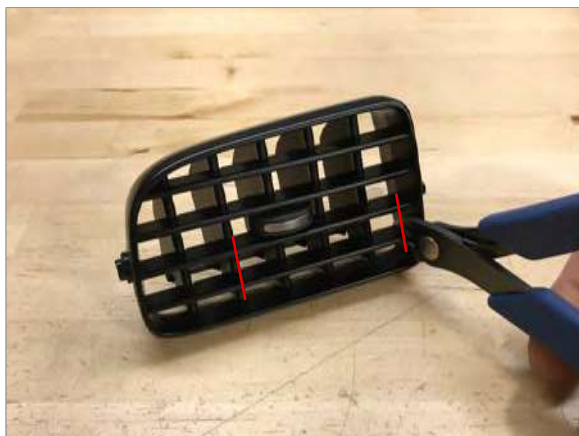
4 Use side cuts to remove bottom two slats as shown.
