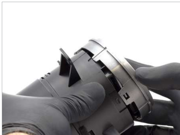
9 Reinstall trim ring onto vent housing.
