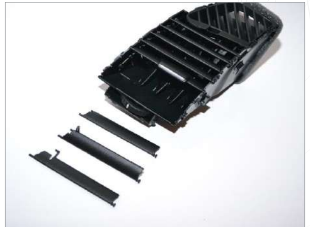
4b Remove the top of the vent completely
