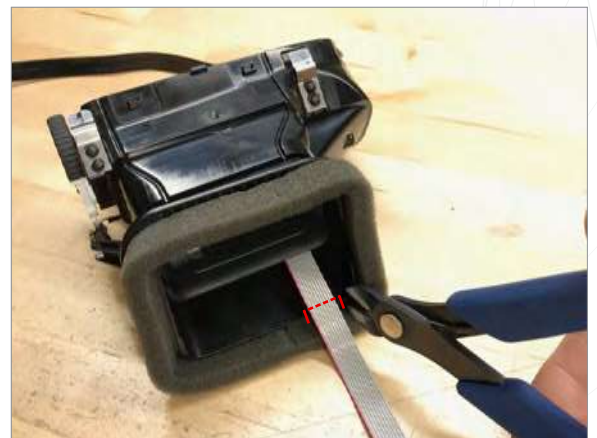
10 Cut relief for ribbon cable in back of vent.
