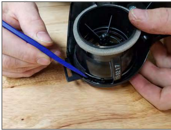
6a Release clips to remove vent from dash trim
