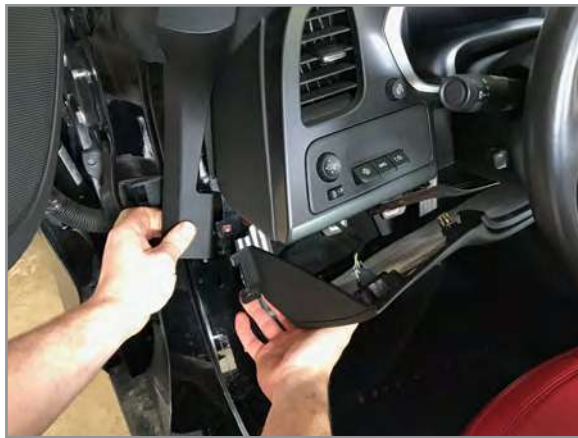
11 Pull lower dash away to gain access to screw
