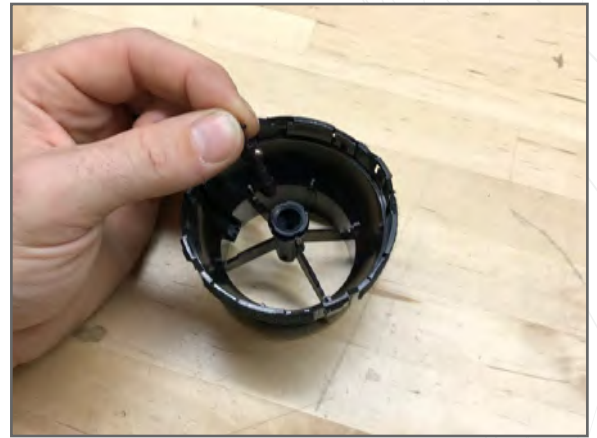
7c Remove center shaft from front of housing
