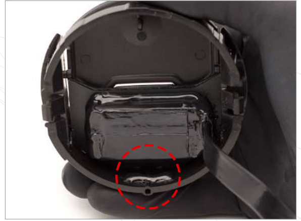
7 (optional) apply glue to bottom two tabs of the display
