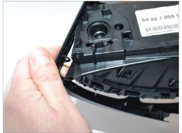
3b Remove the top of the vent completely
