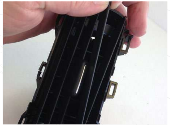
8 While leaving the first vent slat free on the left remove the second vent slat.
