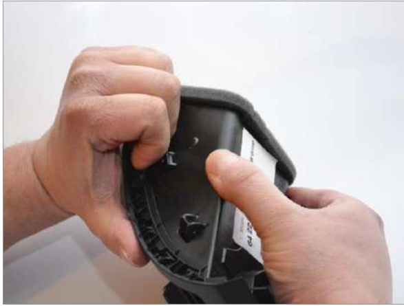
1 Unclip the vent starting on the top right side.
