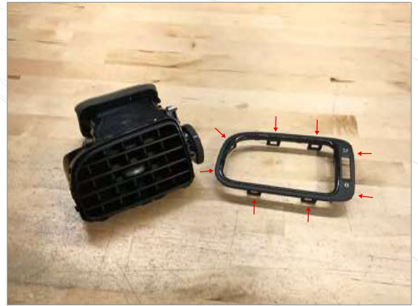
2 Use a small screwdriver to release 8 clips holding trim piece to housing.
