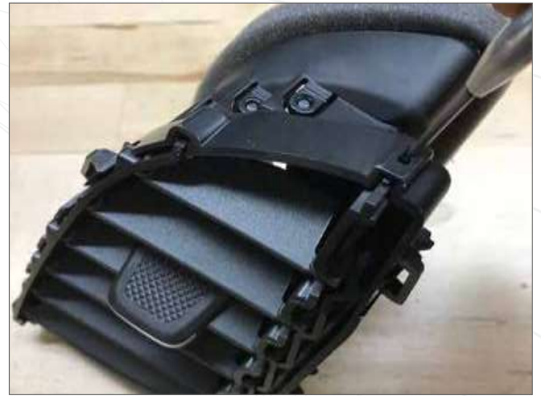
2 Use a small screwdriver to remove vent slat assembly from vent housing.
