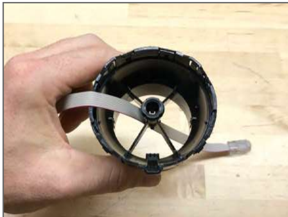
8 Feed display cable through housing as shown
