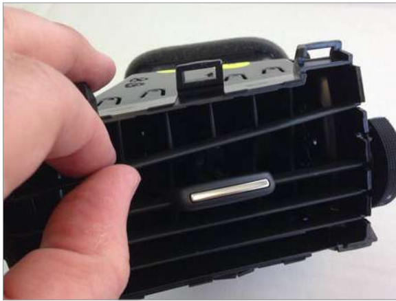
9 Once the second vent slat is out pull the top slat downward slightly as shown to loosen.
