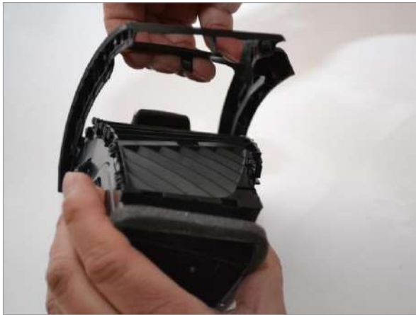
3a Remove the top of the vent and pivot it forward, and then (3b) unclip the bottom circular tabs.
