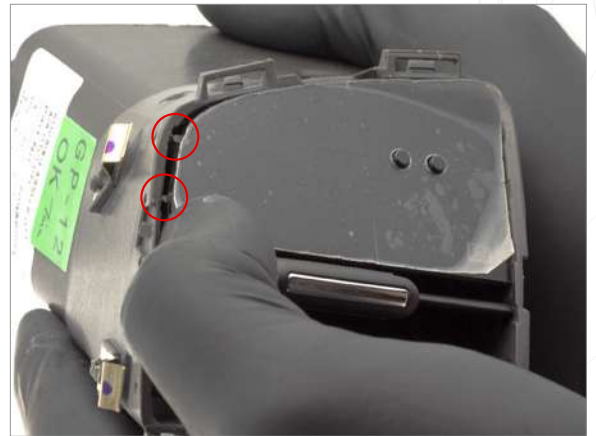
6 Gently push display toward right side of housing and slide left side pins into place.
