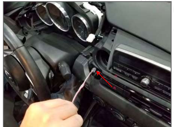
10a Feed display ribbon cable through dash as shown (See 10b)
