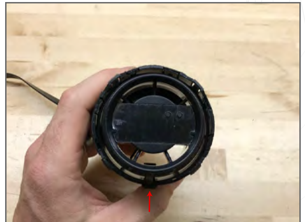
9 Seat display in vent housing (slot shown should in 6 O'clock position when installed in vehicle)
