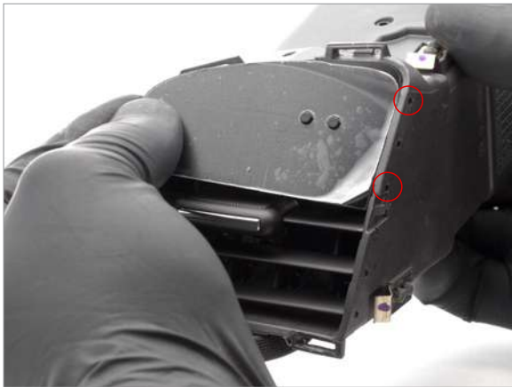
5 Align right (longer) tabs with holes in vent housing and slide into place.
