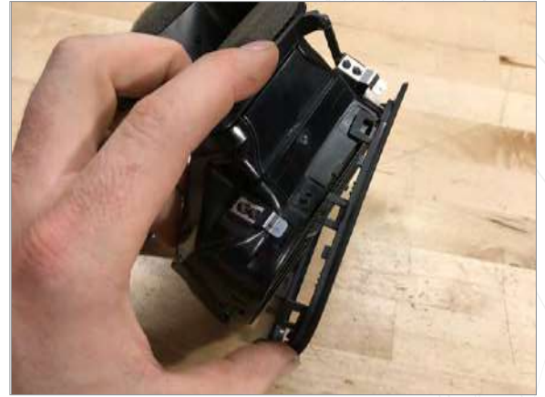
13 Reinstall trim on to vent housing.
