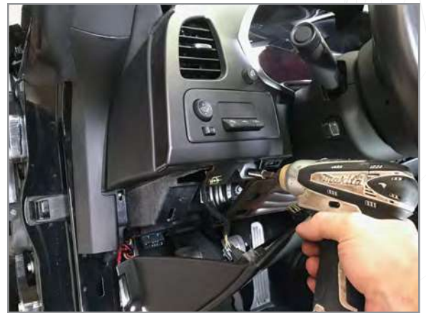
12 Remove dash trim screw as shown
