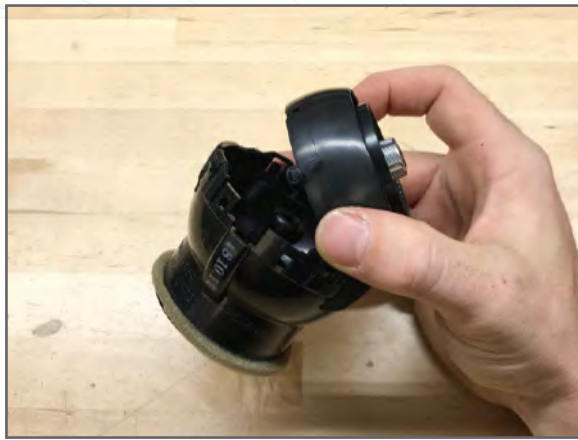
6 Remove slat assembly from housing
