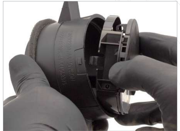
8b Install vent face back into vent housing. Be sure that detent pin stays in position.
