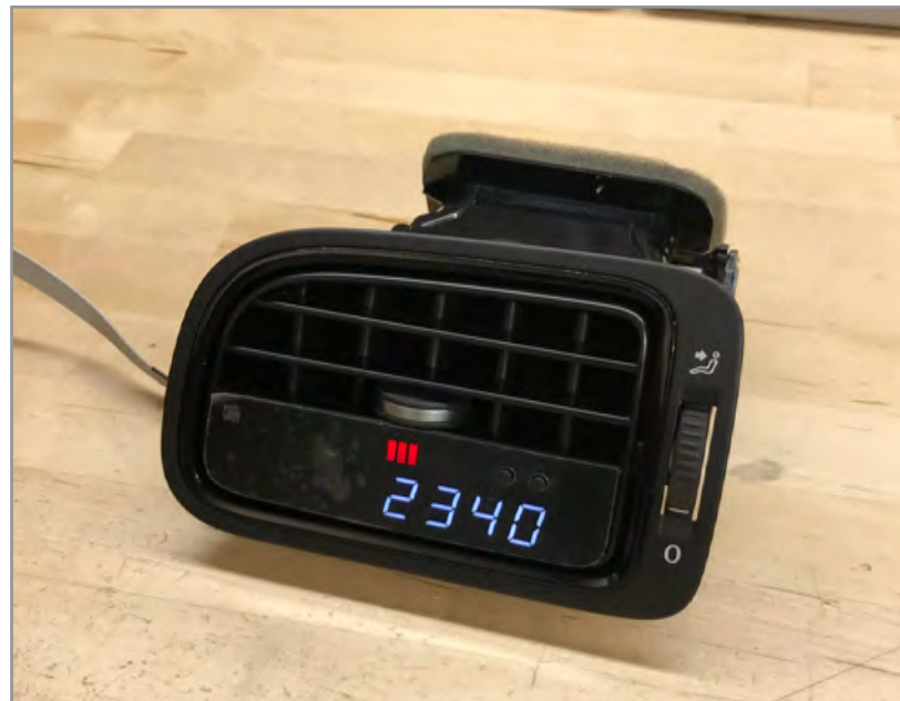
12 Reinstall slat assembly into vent housing.
