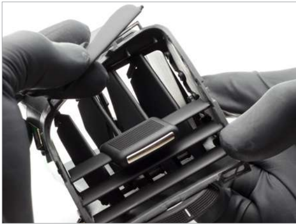
3 Remove stationary slat from vent housing.
