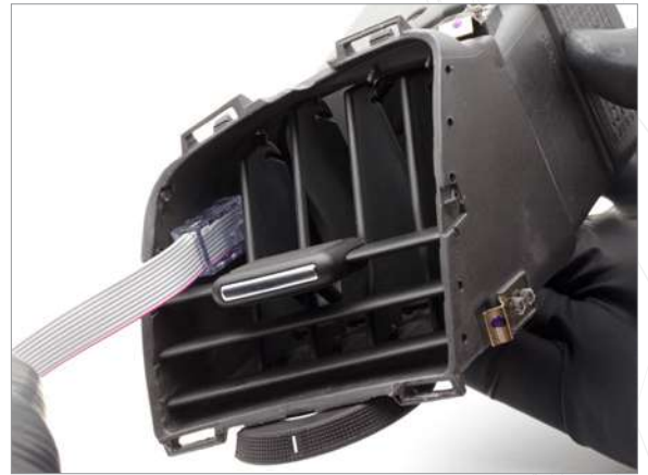
4 Feed display cable to left of vertical slats as shown.
