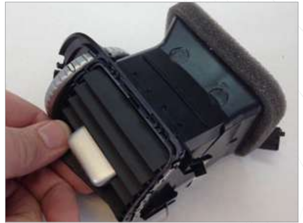
10 Remove the bottom horizontal vent slat.
