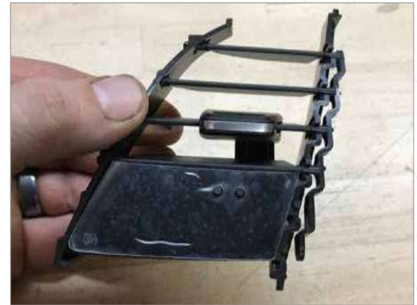
5 Install display into assembly ensuring that pegs on the display are in the vent slat holes on the assembly.
