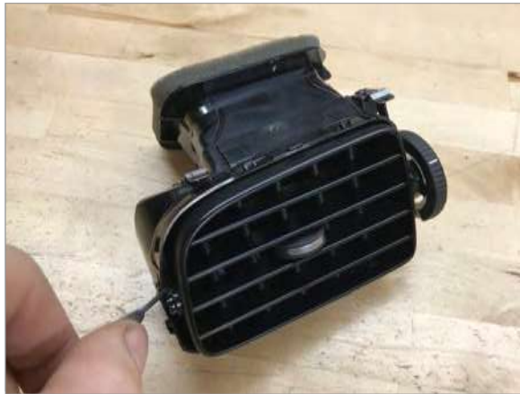
3 Use a screwdriver to remove vent slat assembly from vent housing.
