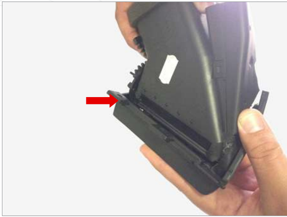
13 Clip front of vent back on rear making sure all seams line up and that lower outer clip is not tucked inside rear of vent housing.
