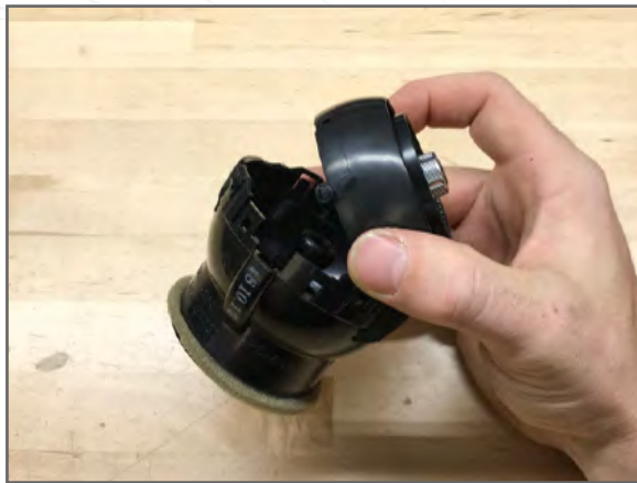
6 Remove slat assembly from housing
