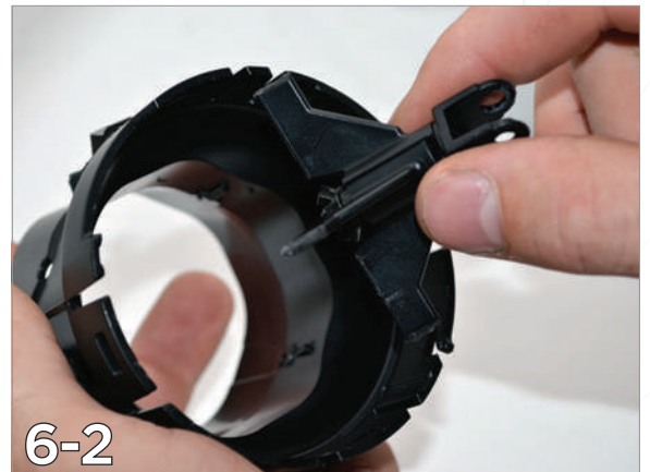
6 Cut the 4 points where the frame connects to the housing and remove the frame.
