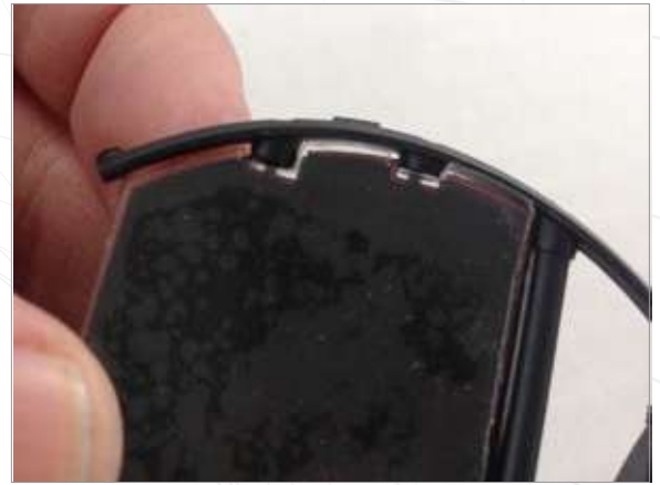
8 Insert the VIDI display into the retainer clip on the left.
