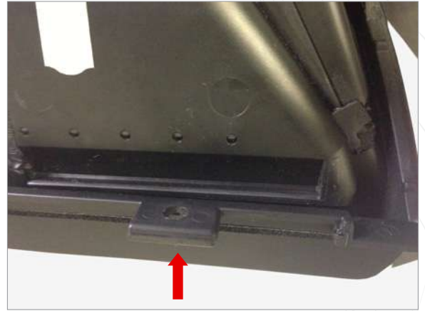
16 Re-attach the vent face, starting at the bottom with the 2 circular clips.
