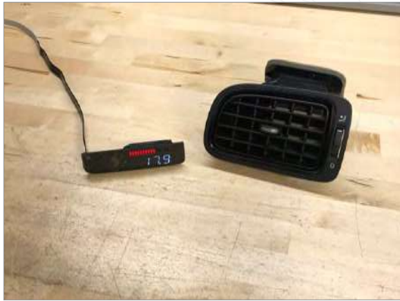
1 Remove vent from vehicle.
