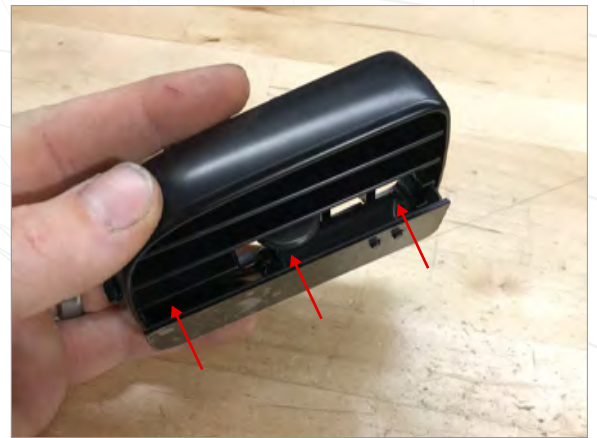
6 Install display into slat assembly ensuring that tabs are lined up correctly
