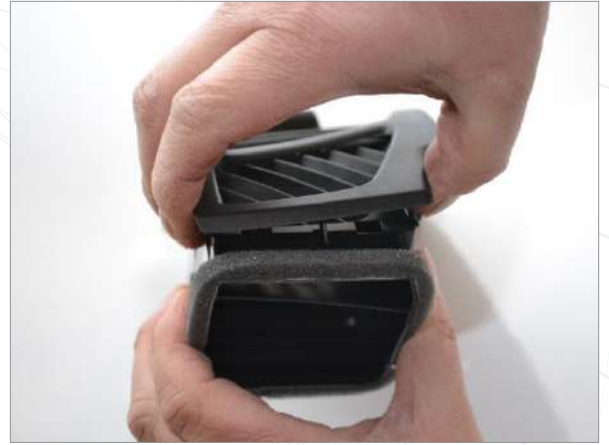
2 Unclip the other side of the vent and pull it away, taking care to unclip the center clip in the middle of the vent.
