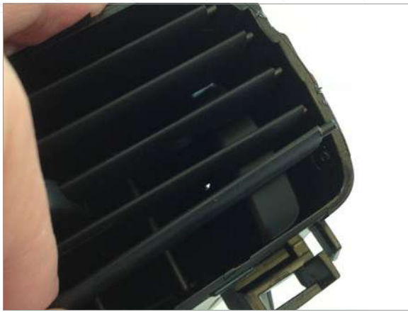
7 Starting with the left side loosen the top vent slat.
