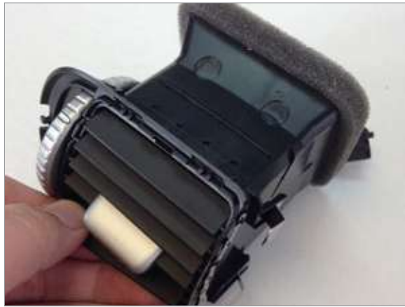
9 Remove the next to last horizontal vent slat.
