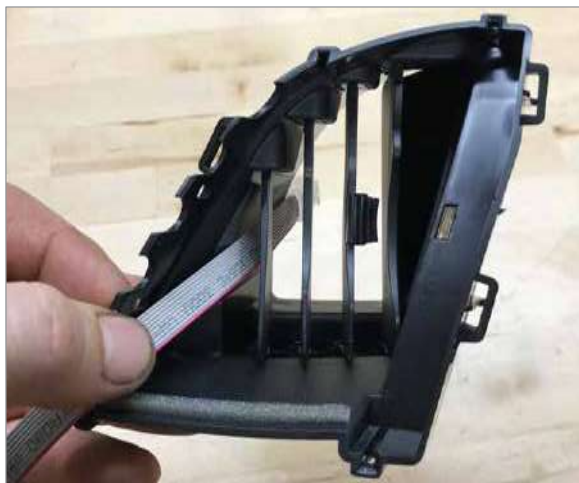
6 Feed display cable through vent as shown.
