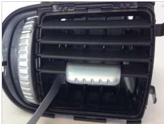
11 Feed in the display cable between the left most wall of the vent housing and the left most vertical vent slat as shown.
