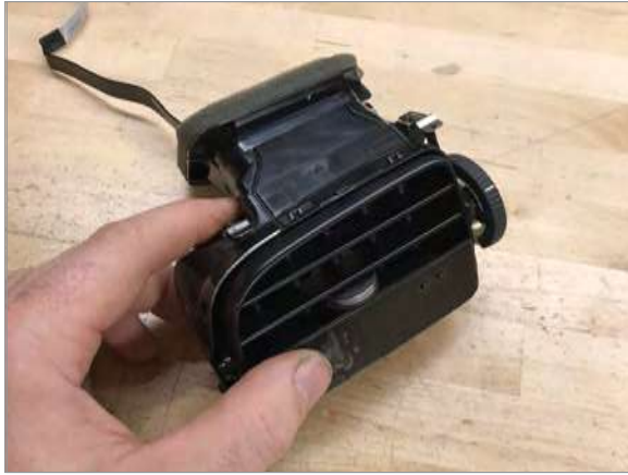
12 Reinstall slat assembly into vent housing.
