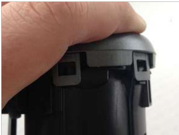
11 Reinstall the trim fascia ensuring clips make firm positive contact.
