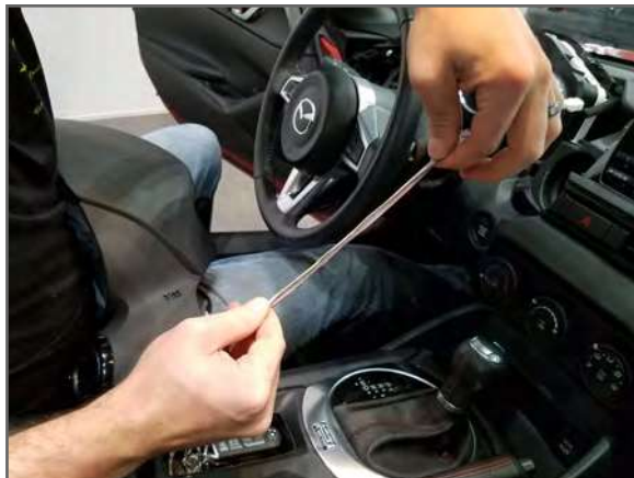
9 Fold display ribbon cable as shown to help feed it through dash
