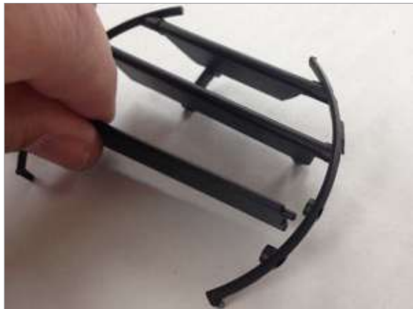
5 Remove the bottom vent slat being careful not to break the plastic.
