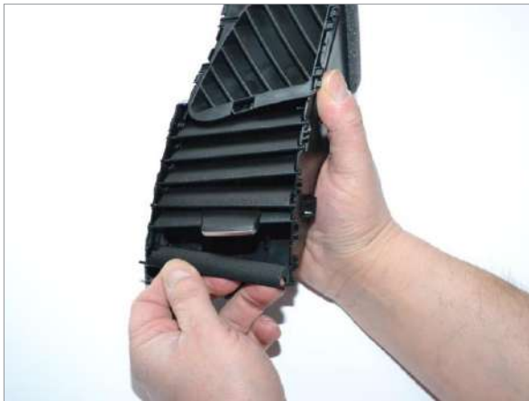
4a Remove the bottom 3 vent slats ONLY.
