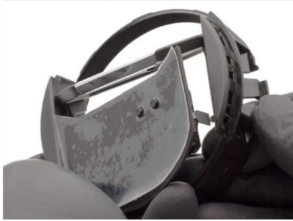
6 Install display into vent face.
