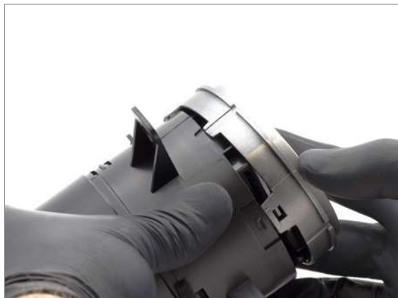
9 Reinstall trim ring onto vent housing.
