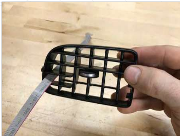
5 Feed ribbon cable through slats as shown.
