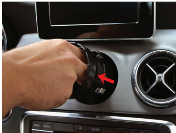
4 With a firm pull, remove the housing from the dash trim.
