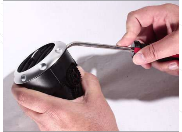
2 when prying off trim ring be sure to keep as much force as possible to the inner most area of the trim ring.
