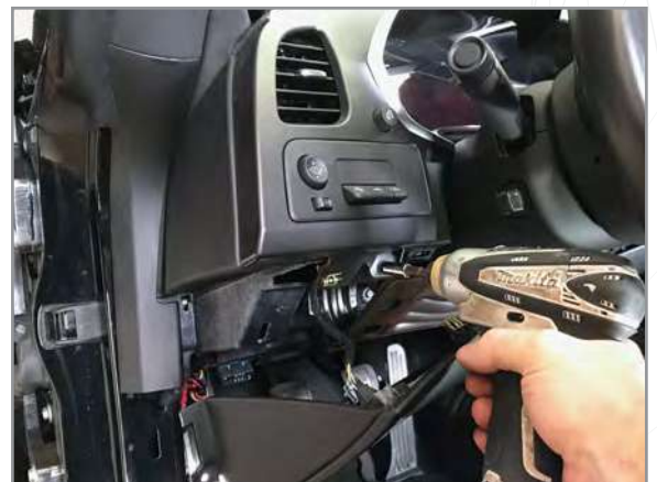
12 Remove dash trim screw as shown
