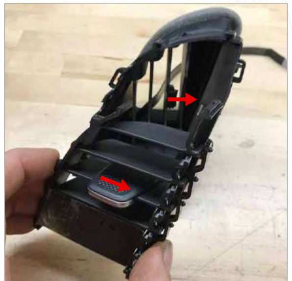
7a Make sure both handle and slats are both pushed as far to the right as possible while assembling.
