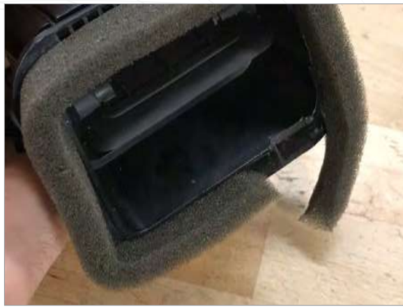
10b Pull foam away from vent as shown.
