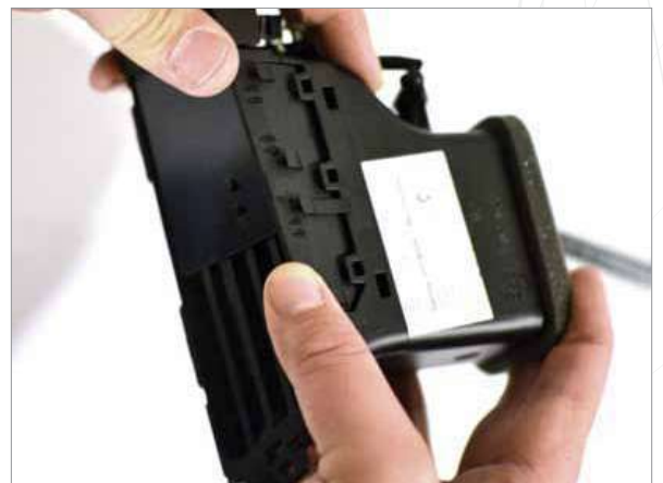
7 Re-attach the vent face. BOTTOM FIRST , after clipping the bottom side, then clip in the top.
