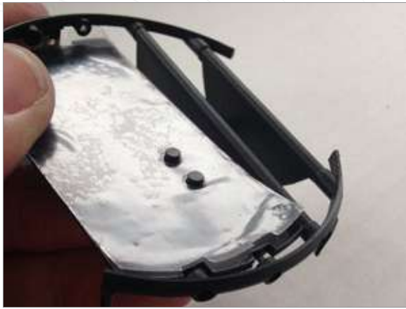
7 Insert the VIDI display right side first.
