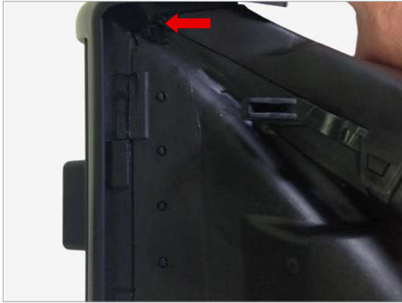
15 With an hi temp epoxy re bind the front and rear of vent housing at union joint.
