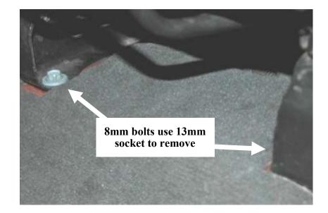
Slide drivers seat back to access the front seat bolts. Remove the front bolts with a 13mm socket on ratchet.
