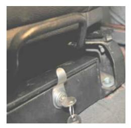
With both front bolts removed slide the drawer unit under seat base so that the tabs with slots of the drawer are under the driver seat front, then replace the two 8mm bolts removed earlier. Tighten the bolts making sure the bolts are down through the driver seat base and through the slots of the drawer unit.
