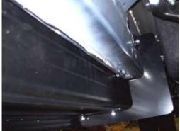
Place the board on the brackets with bolts through slots. Attach with 1/4" nuts loose.
