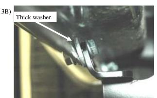
On vehicles produced after July 2015 Chrysler has added a reinforcement bracket on the driver side front location. Install with re-enforcement nut like previously instructed only a thick washer will be placed between bracket and pinch weld as show above.
