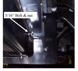
At this time place 5/16" bolt through hole in pinch weld and place nut onto threads. This is done after 1/4" bolts & nut in board are placed into bracket for easier installation of 1/4" bolt into slots of brackets.
