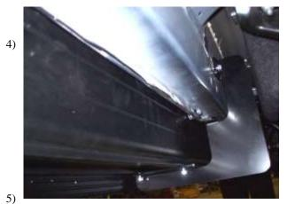
Attach brackets to vehicle by inserting the reenforcement nut in the factory obround hole and leave out the 5/16" bolt and nut through the pinch weld at this time.
