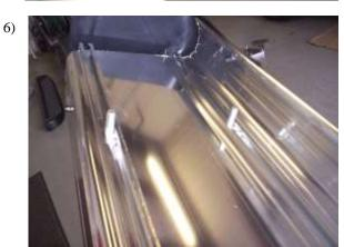
Insert one square head bolt into track for each bracket.
