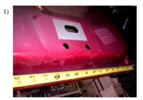
Measure from front wheel well back and : Std Cab—9 1/2" & 54" Quad Cab—9 1/2", 46 3/4", 74 3/8" Crew Cab—9 1/2", 46 3/4", 83 1/4"
