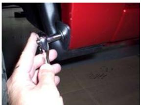
Remove the small factory stone guard in the front fender well by removing the small screw and then unsnap. Reinstall the screw.
