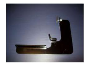
Assemble brackets as shown using one long 5/16" bolt and steel re-enforcement nut. (FL511 shown)
