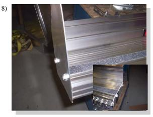
Attach stone guard and end cap to running board using 3/8"self threading bolts.
