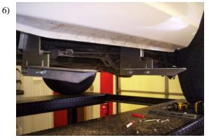
Attach a 3124F angle bracket to the FL185, and attach 3124G (the longer one) to FL175D/P with 5/16" bolts and nuts. Snug but do not tighten at this time.
