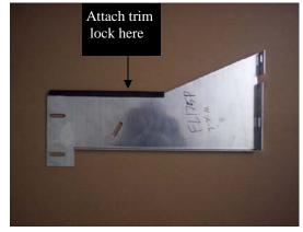
Cut trim lock to 12" and attach to FL175D and P as shown in **Fig 3.**
