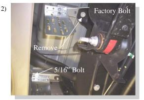
Attach FL73D on bed cross members as shown using 5/16" bolt into inserted clip nut and factory bolt back into fender brace. Use one 3/4" long self drilling screw in each bracket. Remove bed mounting bolt.
