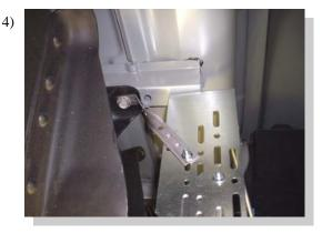
Attach twisted strap using bed mounting bolt removed in step two and one 5/16" bolt and nut as shown.
