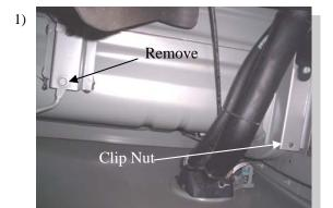
Insert clip nut in forward bed cross member and remove bolt holding fender brace in rearward cross member. (Driver side shown in all photos.)
